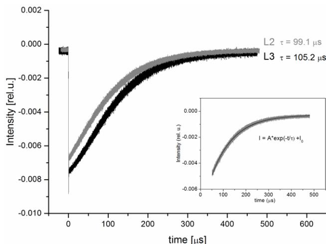
Fig. 5 – Phosphorescence of singlet oxygen as a function of time for L2 and L3 at 25  $\mu\text{M}$  concentration in DCM (The inset shows the fitting procedure with a mono-exponential function).
