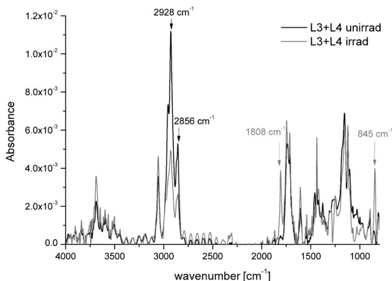
Fig. 6 – FTIR spectra for unirradiated and 1h irradiated solution of L3 (25  $\mu\text{M}$ ) mixed with L4 (25 mM) in DCM.
