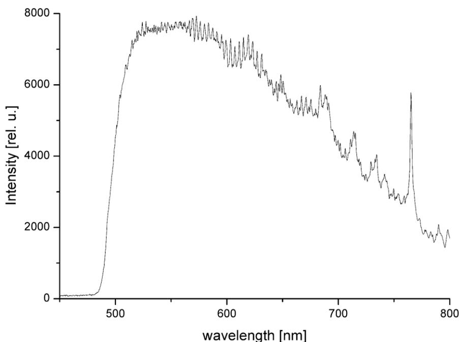
Fig. 2 – Filtered emission spectrum of the Xe lamp.
