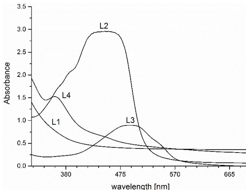
Fig. 3 – Absorption spectra of L1 (50 mM), L2 (100 μM), L3 (50 μM) and L4 (5 mM) solutions in DCM.
