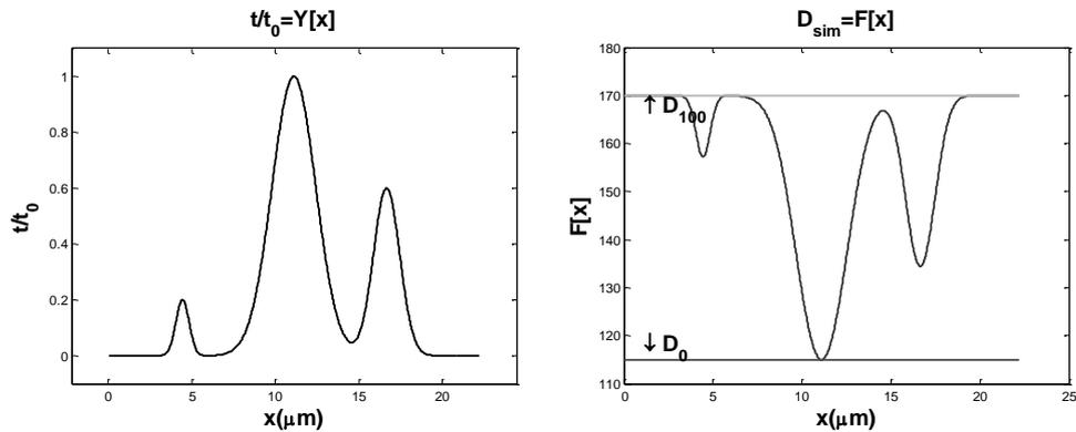
Fig. 4 – A grey level pattern and the exposure dose FTIL reconstruction,  $D_{sim}$ , for a positive EPG 535 photoresist: left – desired relative thickness ( $t_0$  = total thickness of the photoresist); right – corresponding exposure dose ( $\text{mJ}/\text{cm}^2$ ), with  $F(x)$  = exposure dose.
