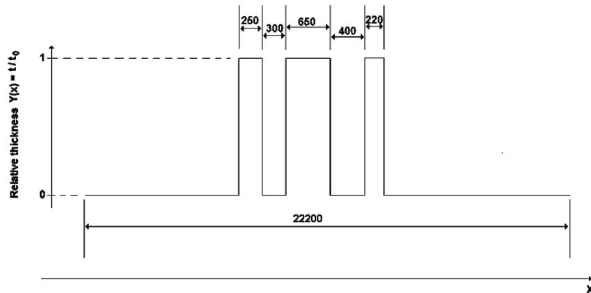
Fig. 5 – The desired photo-resist relative thickness distribution after development (in nanometers).
