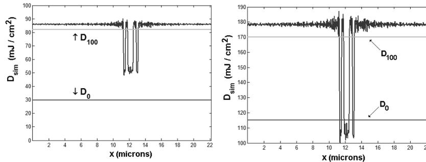
Fig. 6 – The exposure dose FTIL reconstruction for the pattern in Fig. 5 for a positive photoresist: a) the S1813 photoresist; b) the EPG 535 photoresist.
