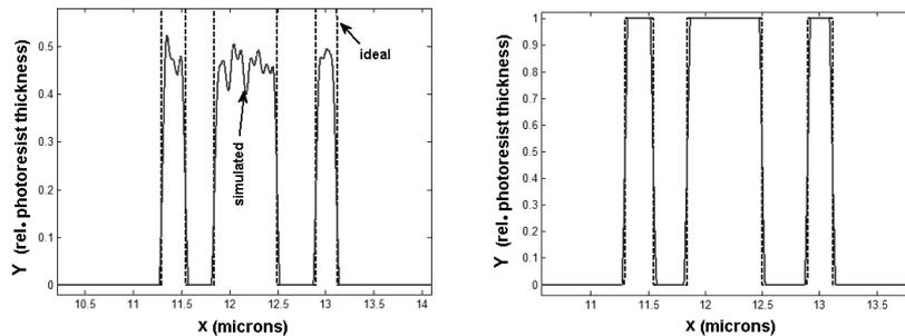
Fig. 7 – An augmented view of the reconstructed region from Fig. 5. The relative thickness of the photo-resist obtained by FTIL reconstruction (continuous line) *versus* ideal photo-resist relative thickness distribution  $Y_{ideal}$  (dashed line), when using a number of  $M = 140$  components; a) refer to S1813 photoresist; b) refer to EPG 535.
