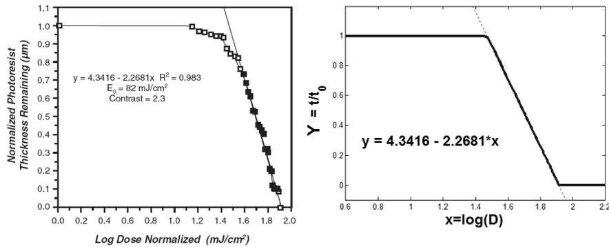
Fig. 3 – The photoresist contrast curve: a) the MICROPOSIT S1813 G2 Photoresist contrast curve [13]; b) idealized response used for simulation.
