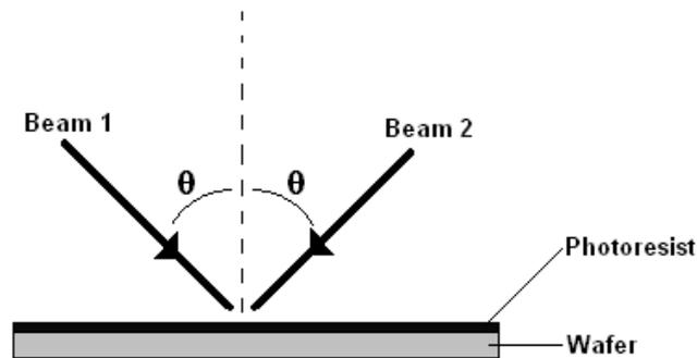
Fig. 1 – The geometry of the interfering beams.
