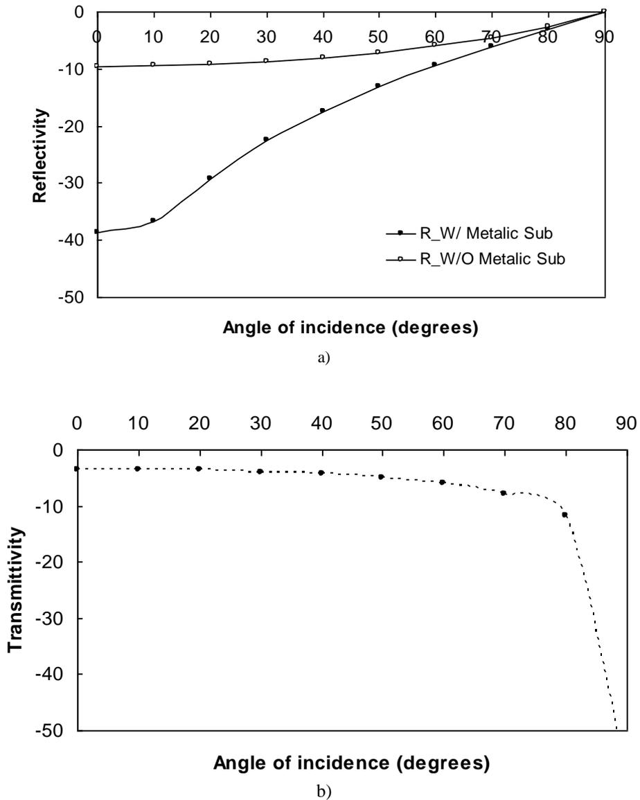
Fig. 6 – a) The reflection with and without the metallic substrate; b) the transmission without the metallic substrate.
