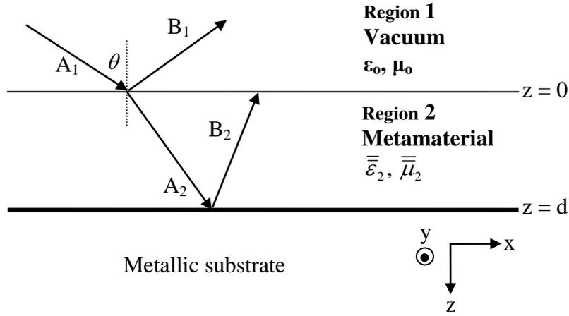
Fig. 1 – Oblique incidence of electromagnetic wave on a metamaterial embedded between semi-infinite free space and metallic substrate.
