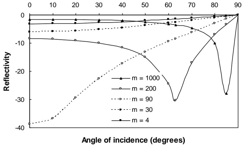
Fig. 4 – The reflection versus the angle of incidence for different values of thickness ( $m = 4, 30, 90, 200, 1000$ ). Here  $\text{Re } \mu = 0$  and  $\text{Im } \mu = 14.3$ .
