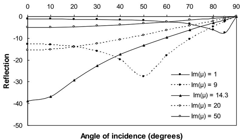
Fig. 2 – The reflection as a function of the angle of incidence for  $m = 90$ ,  $\text{Re} \mu = 0$  and for various values of  $\text{Im} \mu = 1, 9, 14.3, 20, 50$ .
