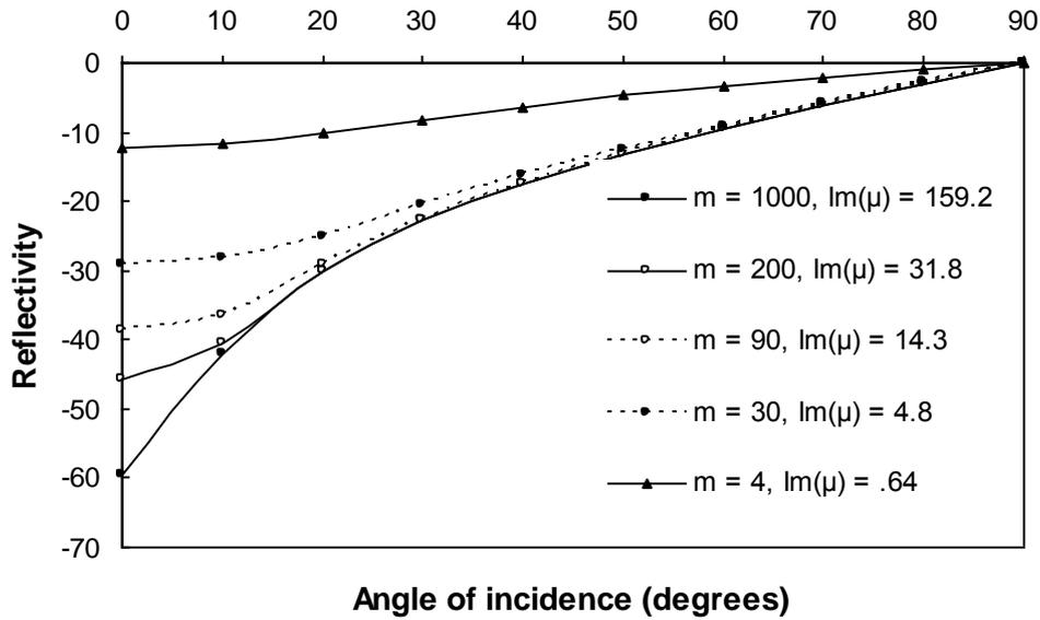
Fig. 5 – The reflection against the angle of incidence for different values of slab thickness ( $m = 4, 30, 90, 200, 1000$ ) and their corresponding values of imaginary part of  $\mu$  ( $\text{Im } \mu = .64, 4.8, 14.3, 31.8, 159.2$ ) with  $\text{Re } \mu = 0$ .
