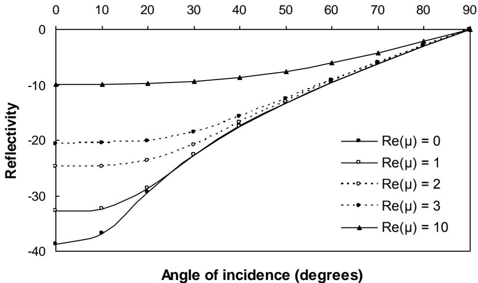
Fig. 3 – The variation of reflection with the angle of incidence when  $\text{Re } \mu$  changes ( $\text{Re } \mu = 0, 1, 2, 3, 10$ ). The values  $m = 90$  and  $\text{Im } \mu = 14.3$  are kept fixed.
