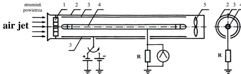
Fig. 4 – Cross-section of a meter measuring the global concentration of air-ions; markings: 1 – coaxial cylinders, 2 – test chamber, 3 – voltage electrode, 4 – collective electrode, 5 – vane, R – height-ohm resistor of the electrometer.
