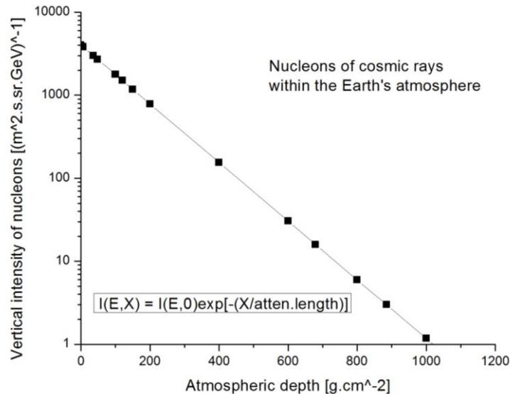
Fig. 2 – Vertical intensity of nucleons at various depth  $X$  in the Earth's atmosphere.
