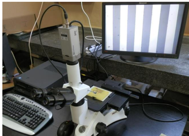
Fig. 7 – The equipment for the analysis of the deposition plates; on screen appears a snapshot of a detail of the deposition plate obtained at 100\times .
