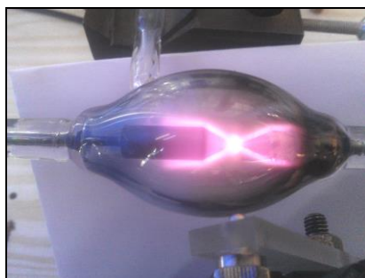
Fig. 1 – Experimental device for the study of bright radiation produced within high-pulsed voltage discharge.
