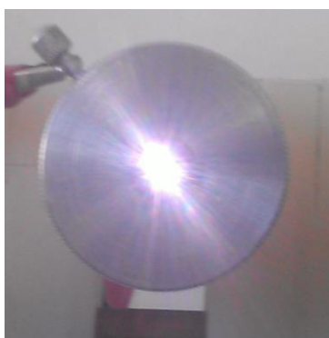
Fig. 14 – Plasma jet image at the outer part of the device.
