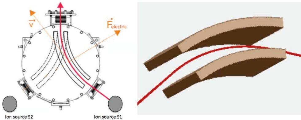
Fig. 3 – Technical drawing (left panel) and SIMION® 8.1 representation (right panel) of LE ESA.
