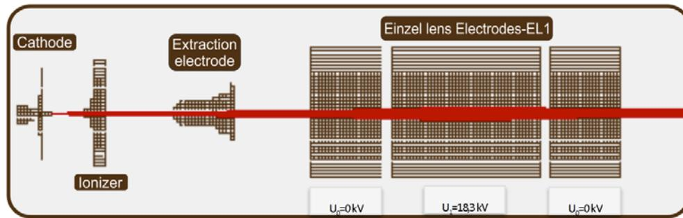
Fig. 2 – 2D simulation of the ion source and the first electrostatic lens (EL1) (SIMION<sup>®</sup> 8.1). The EL1 voltages are obtained from the simulations as given in Table 3.
