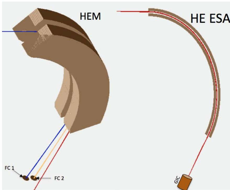
Fig. 6 – Ion Optics simulation of HEM (right panel) and HE ESA (left panel) (SIMION®8.1). FC1 and FC2 are Faraday cups used to measure the ion beam currents.
