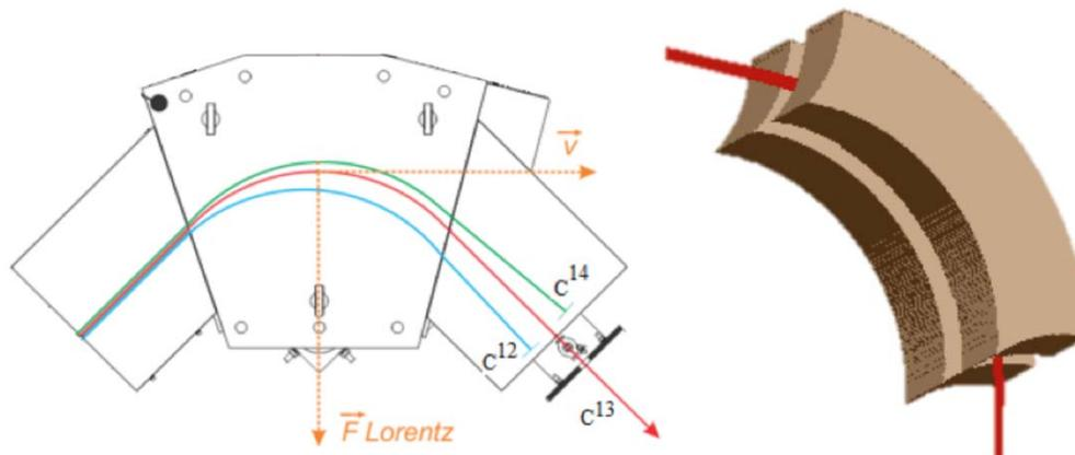
Fig. 4 – Technical drawing (left panel) and SIMION® 8.1 representation (right panel) to the low energy sector magnet (LEM);  $C^{13}$  is the pilot beam and  $C^{14}$  is the “rare isotope” beam.
