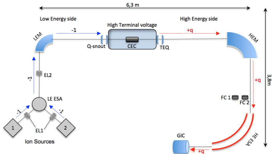
Fig. 1 – General layout of the 1 MV HVEE AMS facility at IFIN-HH, Bucharest, Romania. The symbols “-1/+q” are used to indicate the negative/positive sign of the ion beam charge state. The meanings of the acronyms are given in Table 1.
