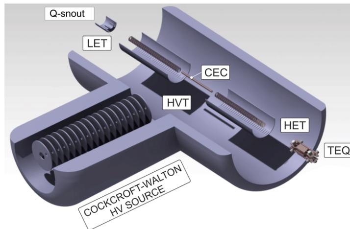
Fig. 5 – 3D layout of the ion optical elements of the accelerator system (CATIA V5); the voltage values for Q-snout and TEQ are given in Table 3 and 4.
