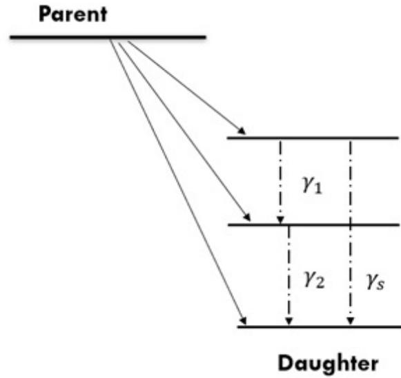
Fig. 1 – Simple gamma cascade decay scheme.
