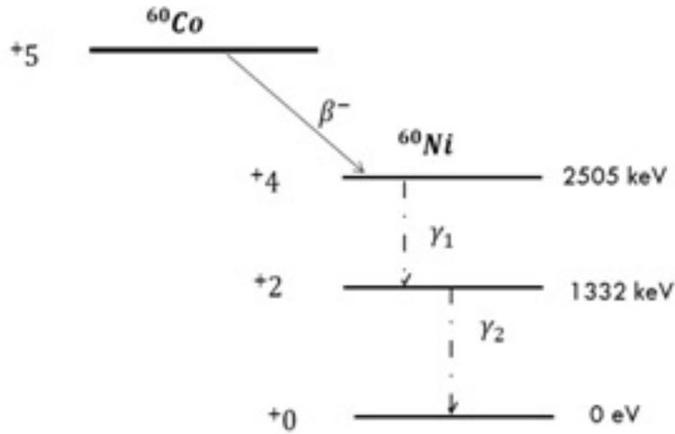
Fig. 2 – Simplified decay scheme of  $^{60}\text{Co}$ .
