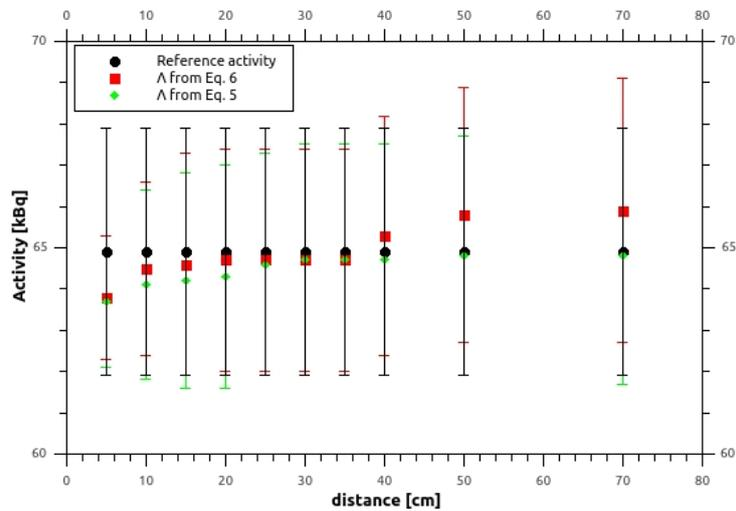
Fig. 3 – The dependence of the calculated activity as a function of the distance.
