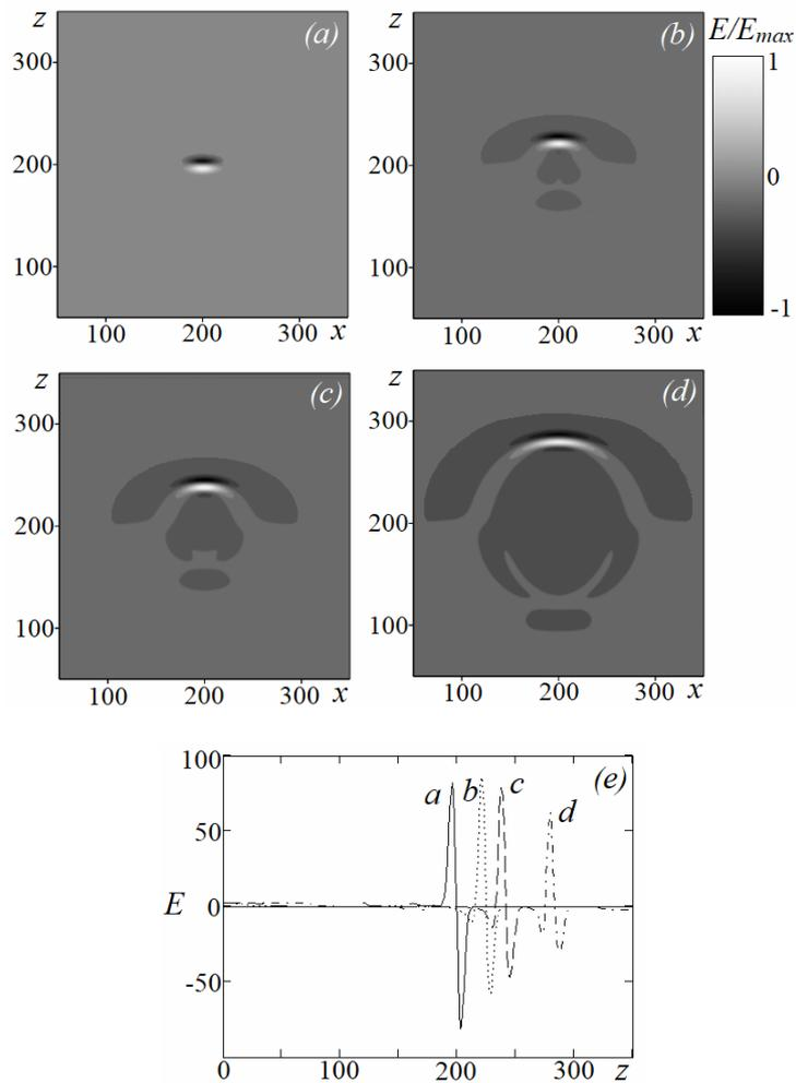
Fig. 1 – The dependence of the electric field on coordinates at different instances of time for initial condition (6a): a) initial pulse; b)  $t = 3 \cdot 10^{-13}$  s; c)  $t = 5 \cdot 10^{-13}$  s; d)  $t = 10 \cdot 10^{-13}$  s; e) the cross-section along the  $z$ -axis.
