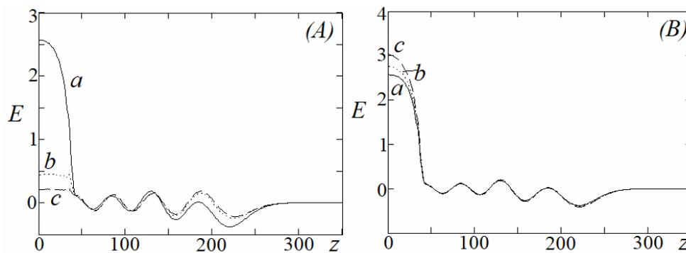
Fig. 3 – The dependence of the electric field of the Airy pulse (longitudinal section) on the coordinate: (A) for different values  $t_{rel}$ : a)  $t_{rel}/t = 5$ ; b)  $t_{rel}/t = 25$ ; c)  $t_{rel}/t = 50$ ; (B) for different values of the gain parameter: a)  $\Gamma = 0.01 \text{ s}^{-1}$ ; b)  $\Gamma = 0.05 \text{ s}^{-1}$ ; c)  $\Gamma = 0.1 \text{ s}^{-1}$ .
