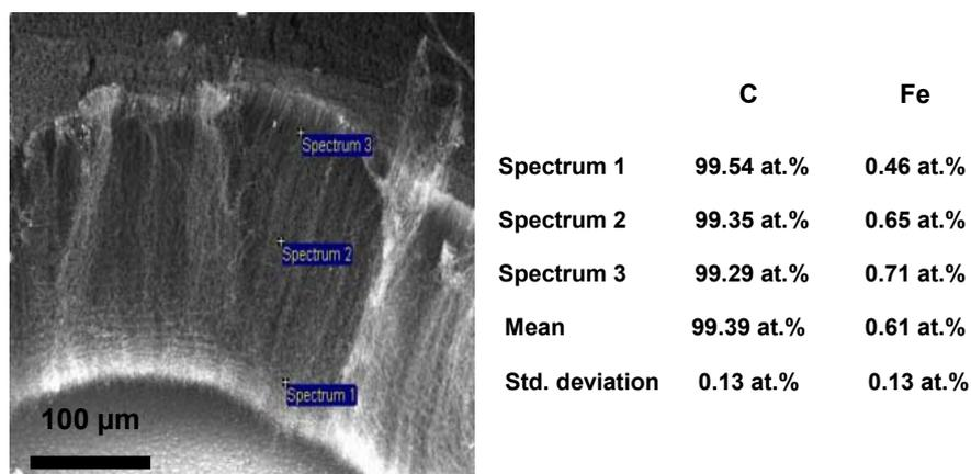
Fig. 2 – EDX analysis in three points along the vertically aligned MWCNT array.
