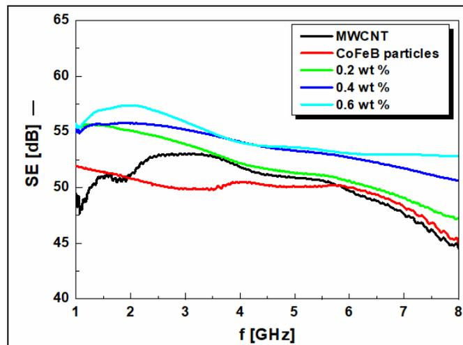
Fig. 5 – Shielding effectiveness (SE) versus radiation frequency for different MWCNTs loadings.
