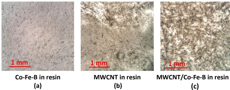
Fig. 4 – Optical microscope images of: a) Co-Fe-B nanoparticles, b) MWCNTs, and c) MWCNTs/Co-Fe-B nanoparticles dispersed in epoxy resin.
