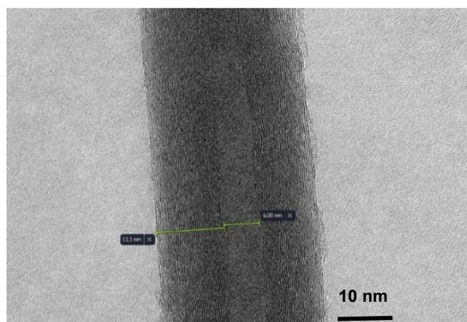
Fig. 3 – HR-TEM image of an individual MWCNT.
