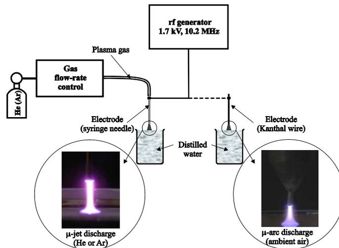
Fig. 1 – Schematic representation of the plasma generator.
