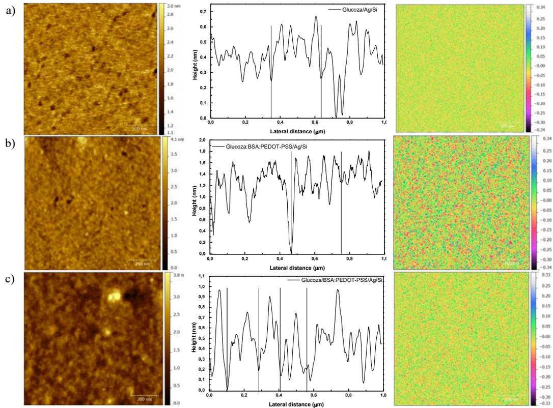
Fig. 4 – AFM records: topography (left), lateral distance (middle) and electrostatic image (right) of a) Glucose/Ag/Si; b) Glucose:BSA:PEDOT-PSS/Ag/Si; c) Glucose/BSA:PEDOT-PSS[1:1]/Ag/Si exposed layers.
