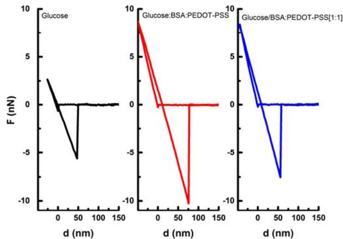
Fig. 5 –  $F(z)$  curves recorded on the active layer's surface of: Glucose/Ag/Si (black), Glucose:BSA:PEDOT-PSS[10:1:1]/Ag/Si (red), Glucose/BSA:PEDOT-PSS[1:1]/Ag/Si (blue) structures (Color online).
