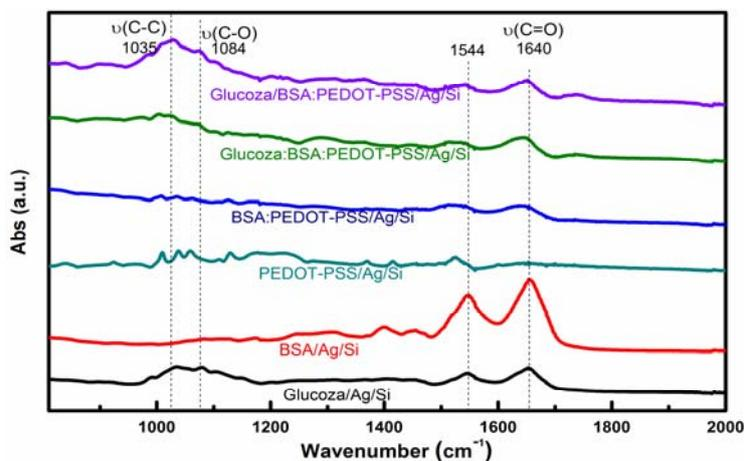
Fig. 3 – ATR/FTIR spectra of Glucose/Ag/Si (black), BSA/Ag/Si (red), PEDOT-PSS/Ag/Si (turquoise), BSA:PEDOT-PSS[1:1]/Ag/Si (blue), Glucose:BSA:PEDOT-PSS[10:1:1]/Ag/Si (green) and Glucose/BSA:PEDOT-PSS[1:1]/Ag/Si (mauve) thin films (Color online).
