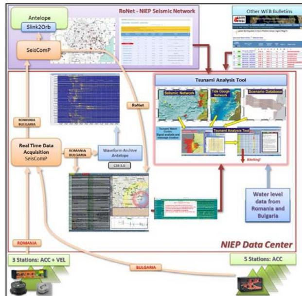
Fig. 9 – Earthquake and tsunami warning system workflow.
