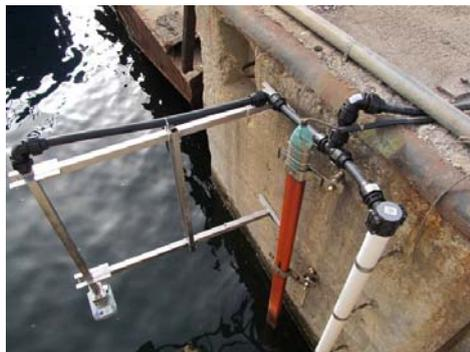
Fig. 2 – The sea level measuring equipment from Constanta port.
