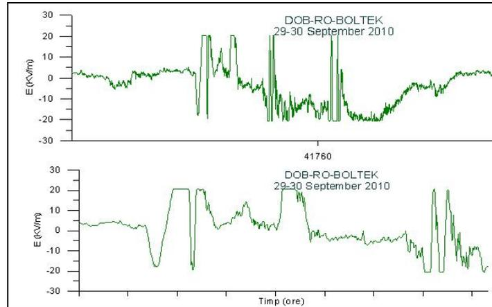
Fig. 8 – Examples of lightning signatures on the electric field recordings.
