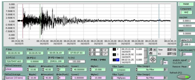
Fig. 13 – P arrival at Mangalia station, for the 15.10.2016 earthquake.
