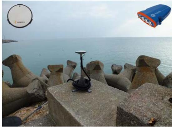
Fig. 3 – GPS/GNSS receiver and antenna located in Mangalia.
