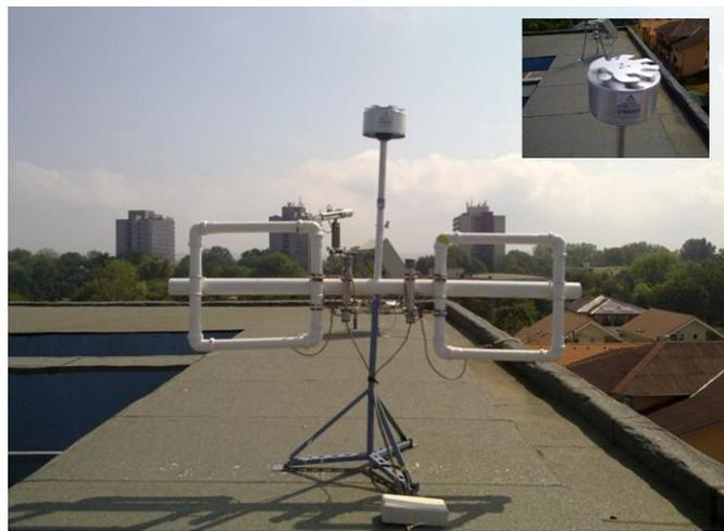
Fig. 6 – The BOLTECK EFM100 electric field mill installed at Eforie Nord.
