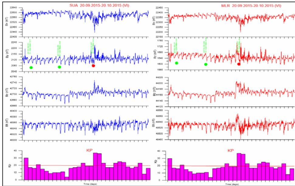
Fig. 2 – (Color online). Anomaly number VI (Table 2) on MLR  $B_y$  component and the earthquakes that occurred during this anomaly and the daily representation of  $K_p$  indices.
