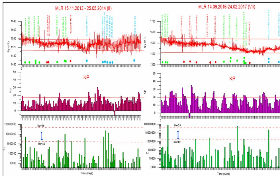
Fig. 4 – Representation of two long-period geomagnetic anomalies (anomaly number II and VII) recorded on  $B_y$  component alongside with the  $K_p$  indices (pink histograms) and the daily seismic energy (green histograms).
