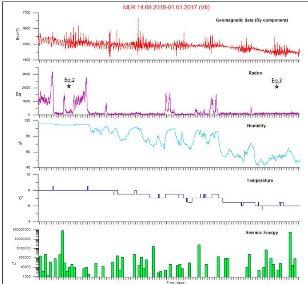
Fig. 5 – Correlation between seismic energy, temperature, humidity and radon readings recorded at MLR observatory during anomaly number VII.
