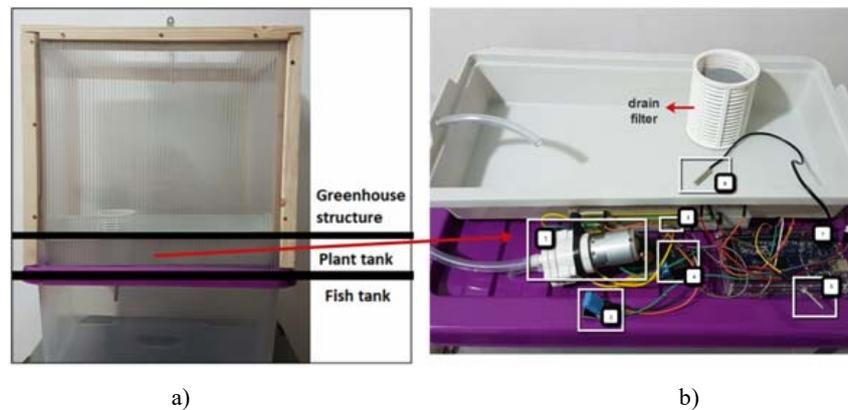
Fig. 8 – The experimental aquaponics system: a) structure of aquaponics system; b) monitoring system 1 – water pump, 2 – temperature and humidity sensor, 3 – resistance 10 k $\Omega$ , 4 – relay, 5 – light sensor, 6 – analog temperature sensor, 7 – Arduino Mega 2560. The colored versions can be accessed at <http://www.infim.ro/rfp/>.
