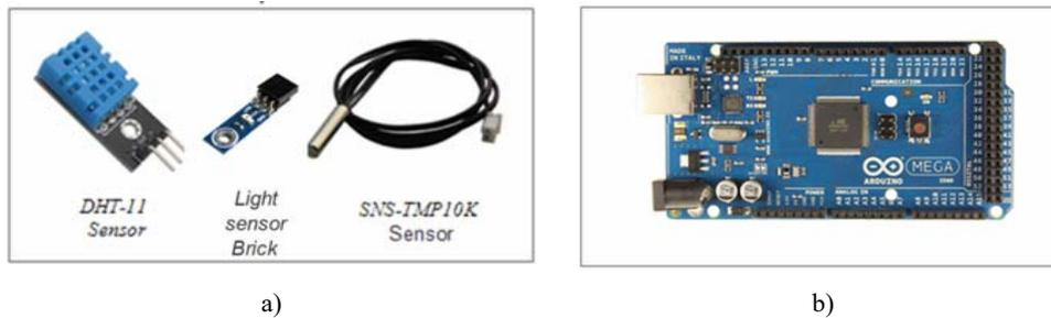
Fig. 3 – Components of the monitoring system: a) Data acquisition unit; b) Arduino unit.
