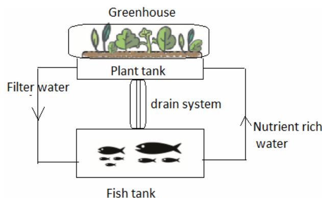
Fig. 1 – The schematic aquaponics system. The colored versions can be accessed at <http://www.infim.ro/rrp/>.
