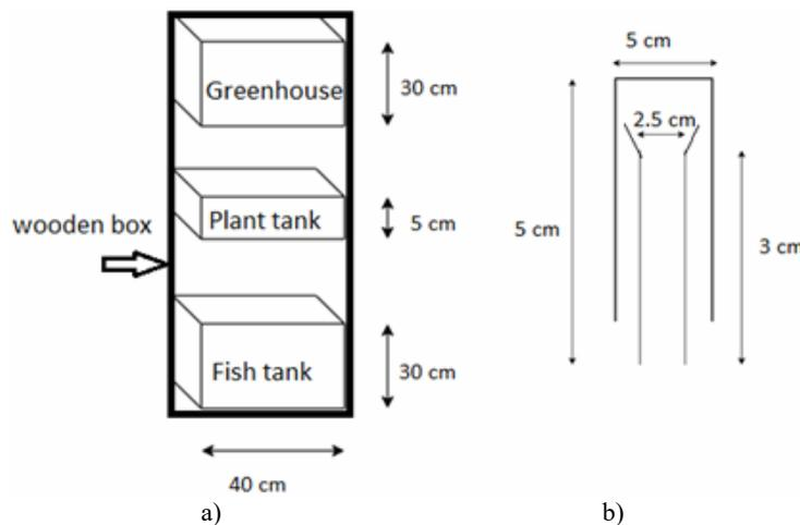
Fig. 2 – a) Aquaponic layer structure; b) drain system.
