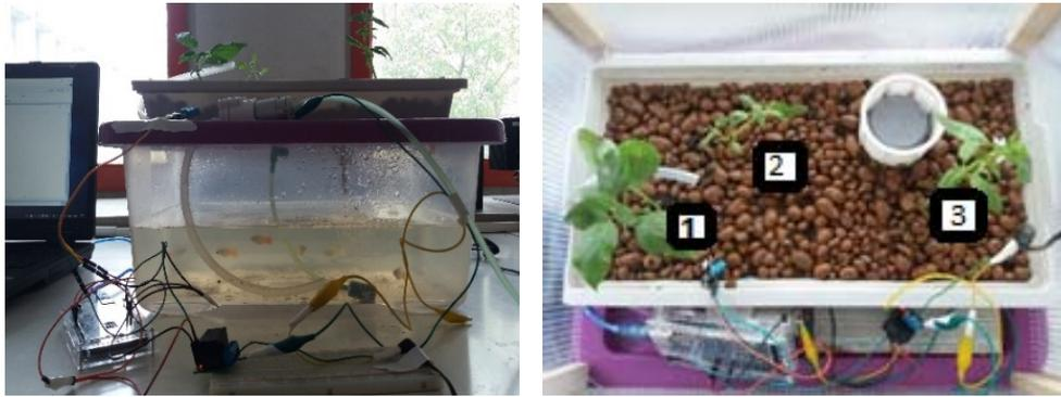
Fig. 9 – The experimental aquaponics system with fishes and plants (basil 1, 2, 3).
