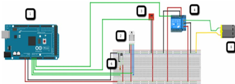
Fig. 6 – Electric scheme of monitoring system: 1 – Arduino Mega 2560, 2 – temperature and humidity sensor DHT11, 3 – light sensor, 4 – 5V relay, 5 – DC motor (water pump simulation), 6 – analogue temperature sensor. The colored versions can be accessed at <http://www.infim.ro/rrp/>.
