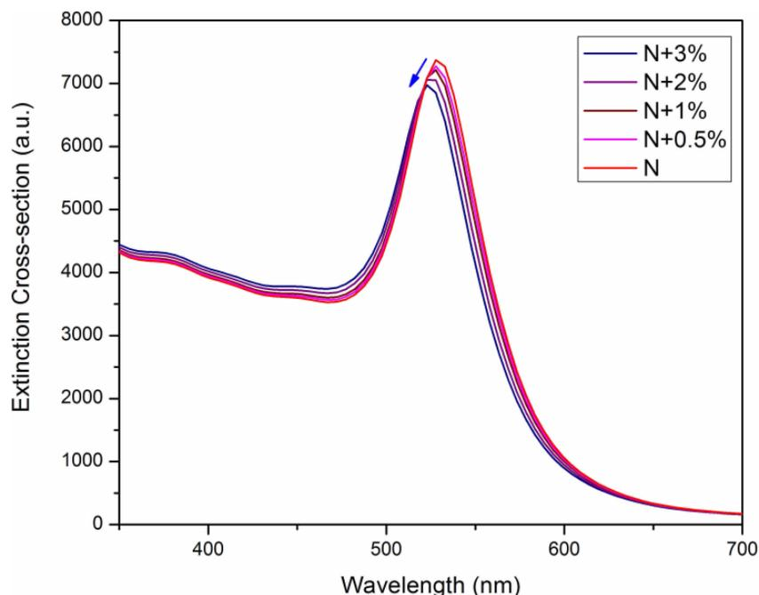
Fig. 5 – Calculated extinction spectra of a 10 nm AuNP for different charge densities. The SPR shifts towards lower wavelengths following an increase in charge density. The shift of the SPR band was lower than 5 nm in the studied interval.
