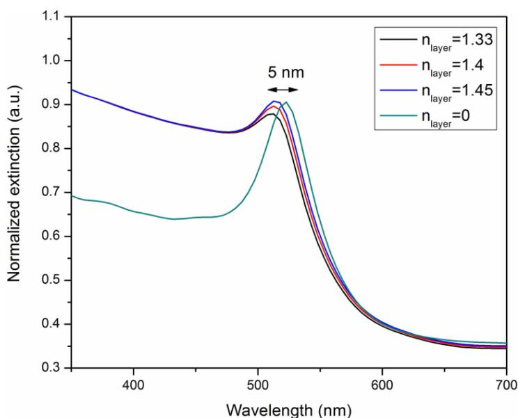
Fig. 6 – Calculated extinction spectra of a 10 nm AuNP using a modified dielectric constant of the surrounding medium, given by the adsorbed  $\text{B(OH)}_4^-$ . The effects of change in refractive index upon chemisorption of  $\text{B(OH)}_4^-$  simulated with a refractive index between 1.33 and 1.45, which leads to a damp of the SPR band, as well as the shift towards lower wavelengths (higher energies). The maximum shift of the simulated SPR band of AuNP is less than 5 nm.
