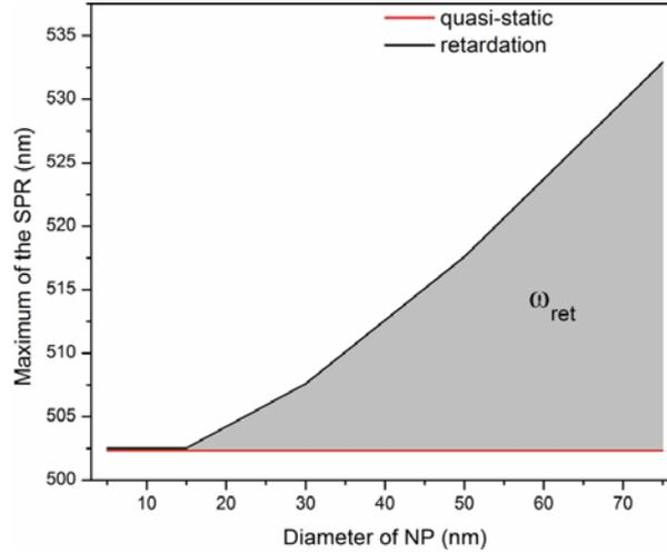
Fig. 4 – Retardation effects on the resonance energy of a AuNP, which depend on the diameter of the nanoparticle, describing the effect of the finite light speed in the metal on the resonance energy.
