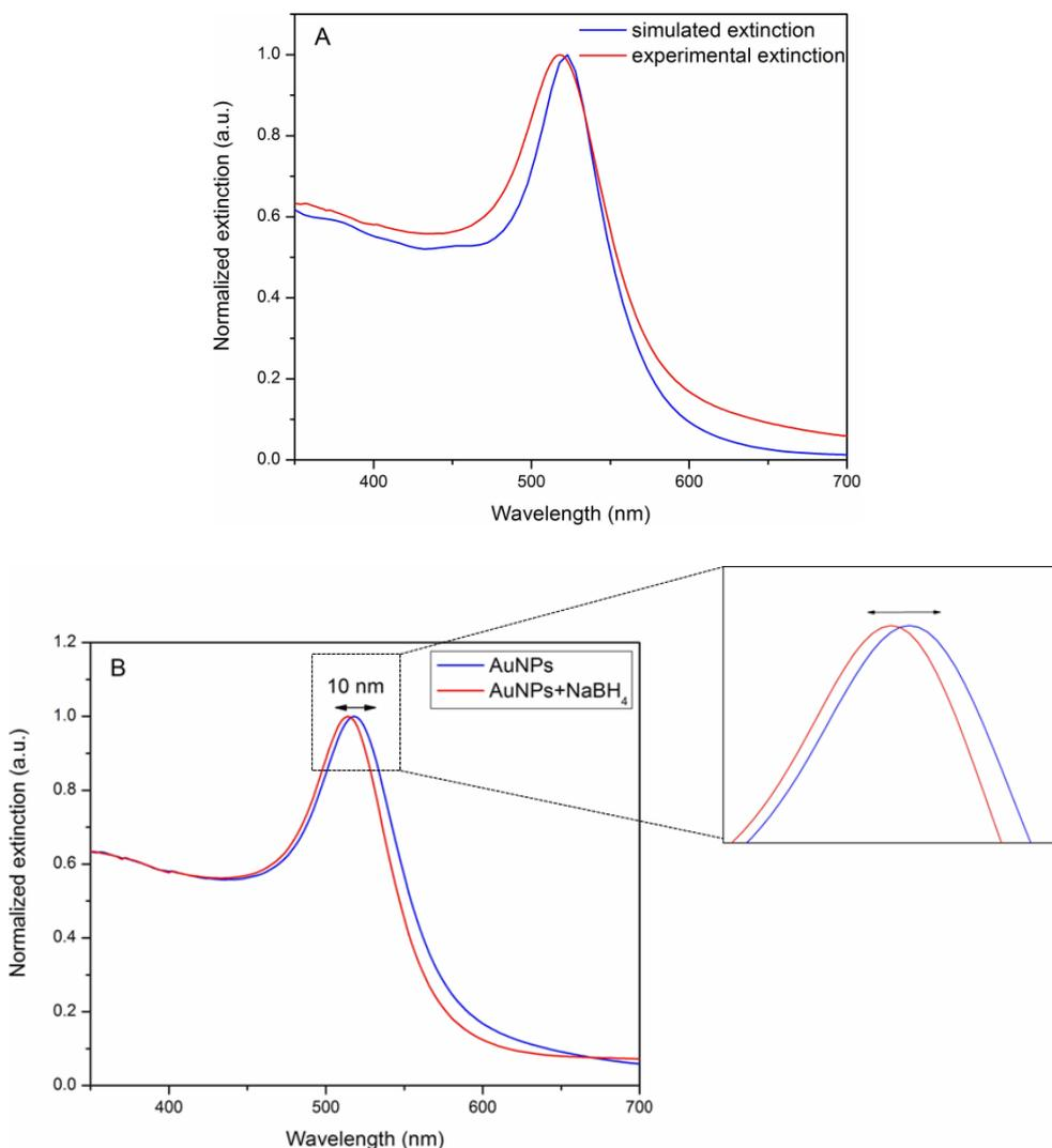
Fig. 2 –A) Simulated and experimental extinction spectra of AuNPs. Three experimental extinction spectra were averaged and both spectra were normalized to unity; B) UV-Vis extinction spectrum of the colloidal AuNPs obtained by citrate reduction and the extinction spectrum of the same colloid after the addition of NaBH<sub>4</sub> 1 mM. The shift of the SPR band of AuNPs upon the addition of NaBH<sub>4</sub> is highlighted in the right image.
