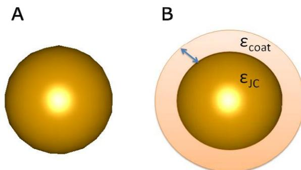
Fig. 1 – Schematic representation of the physical systems used for simulating the optical response of AuNPs: A) gold nanosphere with diameter of 10 nm; B) core-shell system with an inner core of gold of 10 nm diameter and an outer shell of thickness of 1 nm and refractive index determined by the specific chemical nature of the adsorbate.  $\epsilon_{JC}$  represents the dielectric function obtained experimentally [10] and  $\epsilon_{coat}$  the dielectric function of the adsorbate shell.
