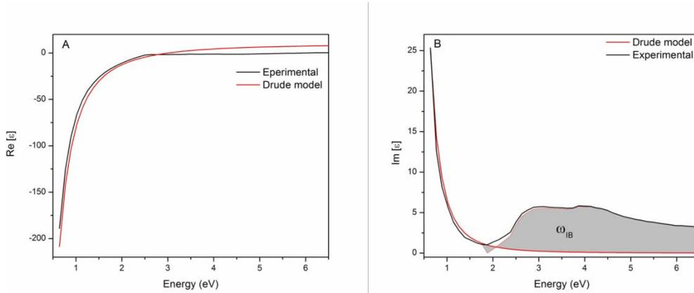
Fig. 3 – The real (A) and imaginary (B) part of the dielectric constant of Au obtained experimentally by Johnson and Christy [10] and simulated on a 10 nm AuNP, based on the Drude model.
