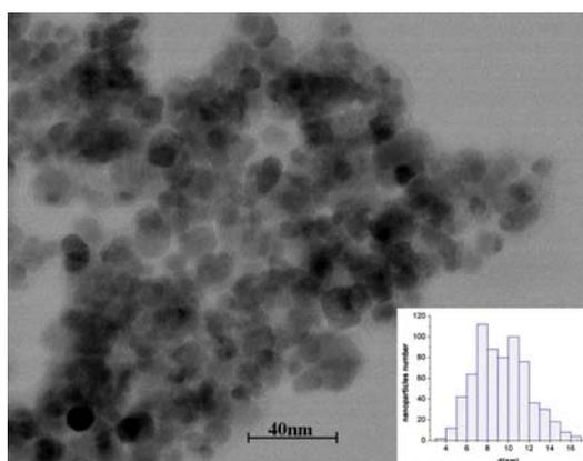
Fig. 2 – TEM image and size distribution of AIONPs (scale bar = 40 nm).
