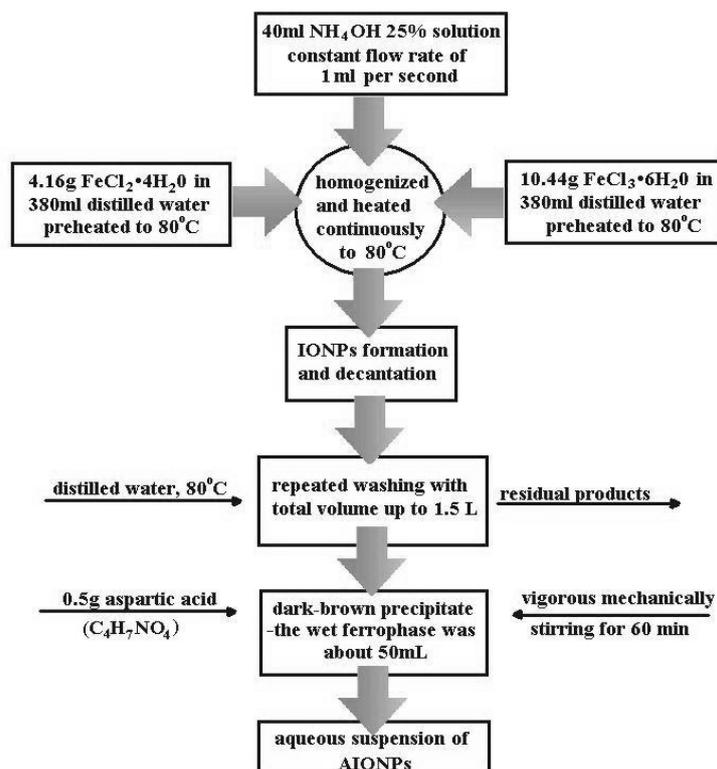
Fig. 1 – Schematic presentation of AIONPs synthesis technology.
