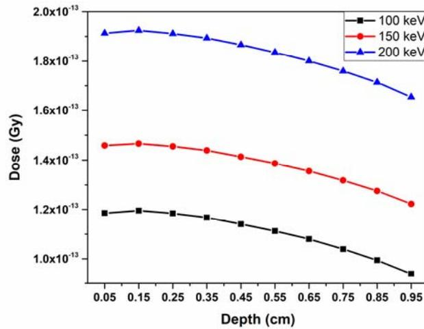
Fig. 3 – The absorbed dose value as a function of depth inside the BK-7 glass sample (straight positioned) for three different gamma-ray energies (100 keV, 150 keV, and 200 keV).
