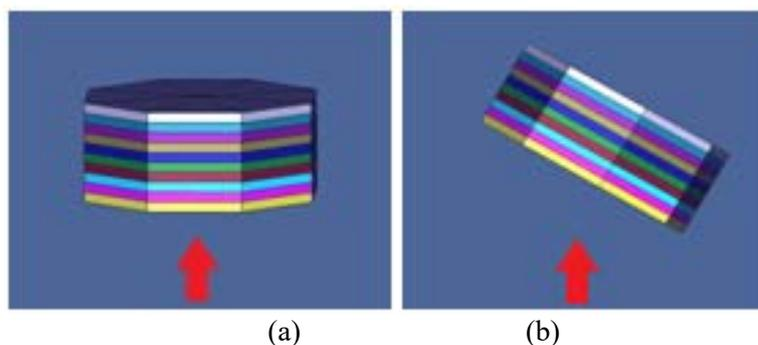
Fig. 1 – The BK-7 cylindrical sample divided into 10 disk-shaped samples to investigate the depth dose distribution into the glass volume (a) straight position, (b) rotated with 45°.
