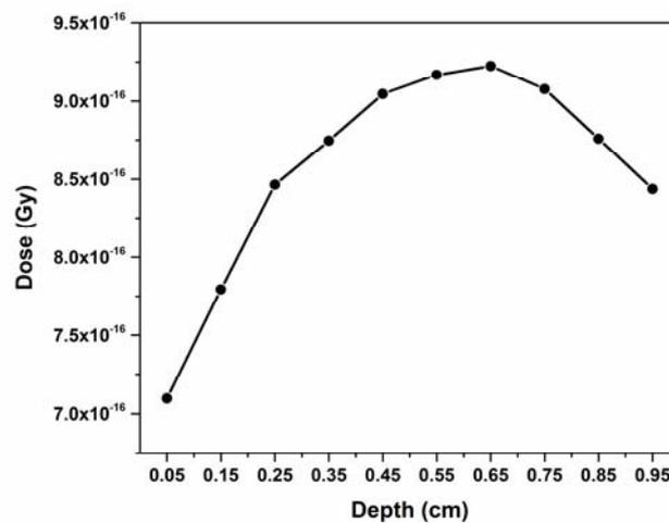
Fig. 4 – Dose value as a function of depth inside the BK-7 glass sample for a 45° rotated sample. The point source is of 100 keV energy.
