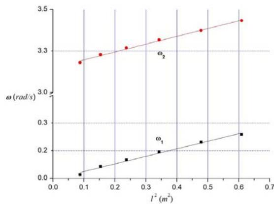
Fig. 8 – Dependence of  $\omega_1$  and  $\omega_2$  as function of  $l^2$  for pendulum 2. For readability reasons, we broke the OY axis. The full color version may be accessed at <http://www.rp.nipne.ro>.
