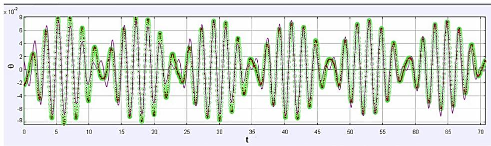
Fig. 6 – Experimental data and fitting plot of the angular elongation as function of time for one of the pendulum illustrating the beats. The full color version may be accessed at <http://www.rpp.nipne.ro>.
