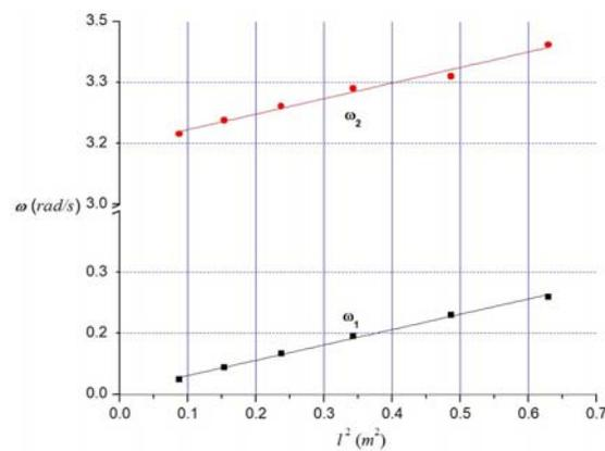
Fig. 7 – Dependence of  $\omega_1$  and  $\omega_2$  as function of  $l^2$  for pendulum 1. For readability reasons, we broke the OY axis. The full color version may be accessed at <http://www.rp.nipne.ro>.
