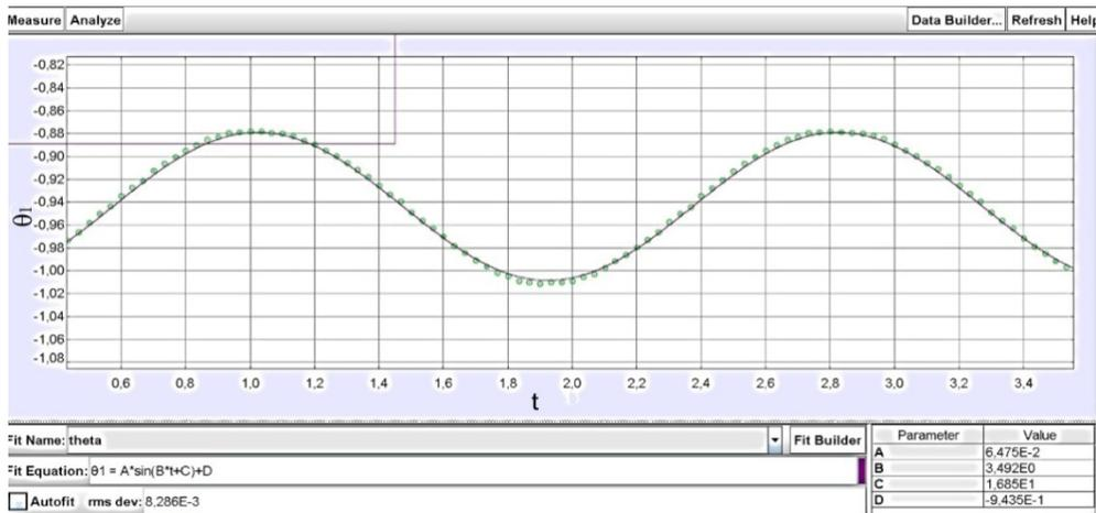
Fig. 3 – Data fitting view of the Tracker software. Experimental and fitted data for angular elongation as function of time, for one of the pendula. The full color version may be accessed at <http://www.rrp.nipne.ro>.
