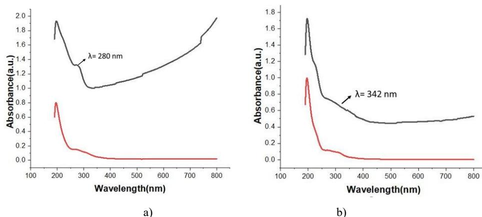
Fig. 5 – Overlapping of the experimental UV-VIS absorption spectra of the water samples from: a) Căldărușani Lake polluted with used cooking sunflower oil (black) and after cleaning with natural absorbent (red); b) Căldărușani Lake polluted with Diesel oil (black) and after cleaning with natural absorbent (red). The full color version can be accessed at <http://www.rpp.nipne.ro>
