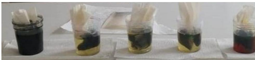
Fig. 1 – Samples of absorbent immersed in each type of oil. The full color version can be accessed at <http://www.rrp.nipne.ro>
