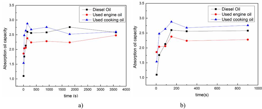
Fig. 3 – Absorption oil capacity as a function of time(s): a) during one hour; b) in the first 900 s.
