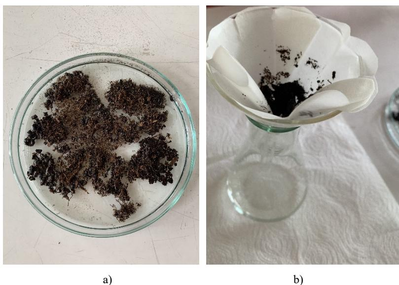
Fig. 2 – Preparation of the samples for UV-Vis spectroscopy: a) immersing the natural absorbent in water and oil; b) the hydrocarbon-soaked absorbent removed by filtration. The full color version can be accessed at <http://www.rrp.nipne.ro>
