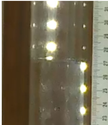
Fig. 2 – Image of the free surface of the water and the “crossing” of the LEDs light images due to the refraction phenomenon. The full color version may be accessed at http://www.rrp.nipne.ro .
