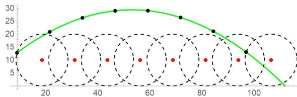
Fig. 4 – (Color online) The ballistic trajectory (green color and black points) and the wheel center (red points) after detaching of  $P$ . Detaching of  $P$  takes place at the black dot with the smallest value of  $x$  coordinate (the leftmost black point), which corresponds to  $\theta_m$ . The parameters of motion are the same as in Fig. 3.
