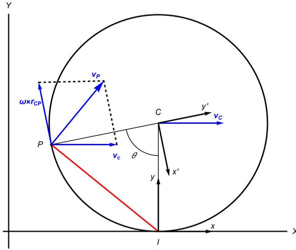
Fig. 1 – (Color online) Rolling without sliding wheel as a planar RB.
