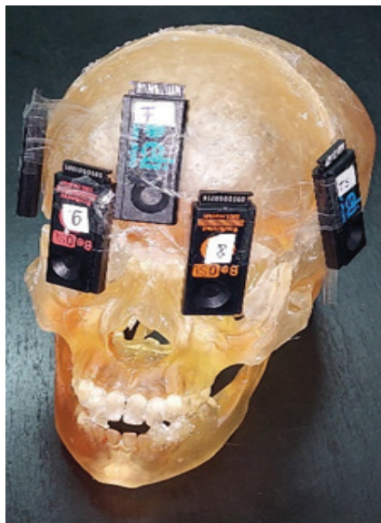
Fig. 3 – The 3D human head phantom equipped with five OSL standard dosimeters.
