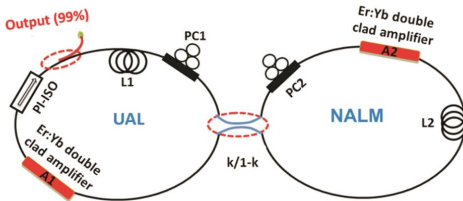
Fig. 1 – Experimental setup of the dual-amplifier figure-of-eight fiber laser.
