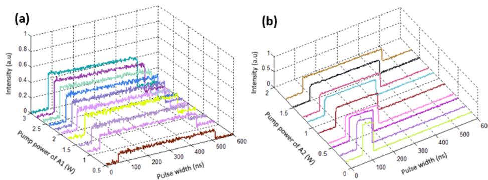
Fig. 2 – Oscilloscope trace of square-wave pulse: a) temporal trace evolution *versus* pumping power of A1; b) temporal trace evolution *versus* pumping power of A2.
