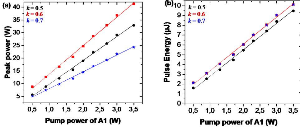
Fig. 3 – a) Peak power and b) pulse energy *versus* pump power of A1 for the different central coupling ratios  $k$  at  $A_2 = 1.8$  W. The straight lines are linear fits.
