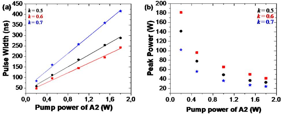
Fig. 4 – a) Pulse width and b) peak power *versus* pump power of A2 for different central coupling ratios  $k$  at  $A_1 = 3.5$  W. The straight lines are linear fits.
