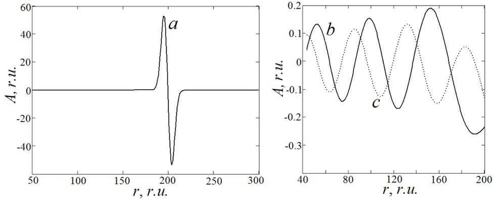
Fig. 4 – A portion of the dependence of the electric field for the Airy pulse on the radius in the direction along the radius: a)  $t = 0$ ; b)  $t = 1 \cdot 10^{-13}$  s; c)  $t = 5 \cdot 10^{-13}$  s.
