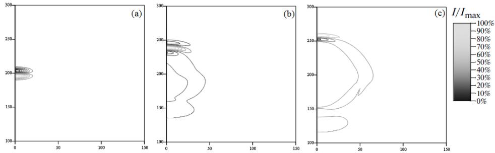
Fig. 1 – The intensity of 3D electromagnetic pulse  $I(r, z, t) = E^2(r, z, t)$  at different values of time: a) the initial pulse shape; b)  $t = 5 \cdot 10^{-13}$  s; c)  $t = 7 \cdot 10^{-13}$  s.
