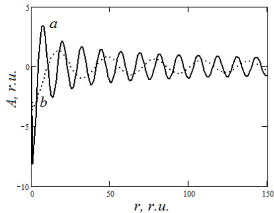
Fig. 3 – The dependence of the electric field for the Bessel pulse on the radius in the direction of the pulse propagation: a)  $t = 0$ ; b)  $t = 5 \cdot 10^{-13}$  s.
