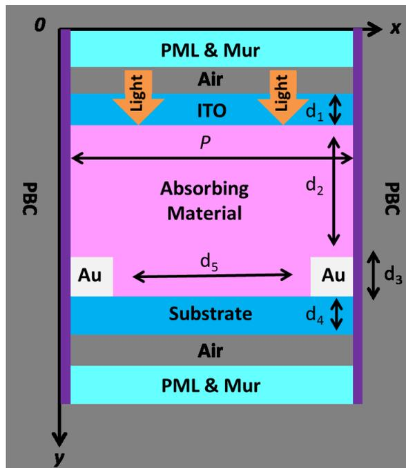
Fig. 1 – Schematic diagram of the unit cell of the plasmonic thin-film solar cell (after Ref. [22]).
