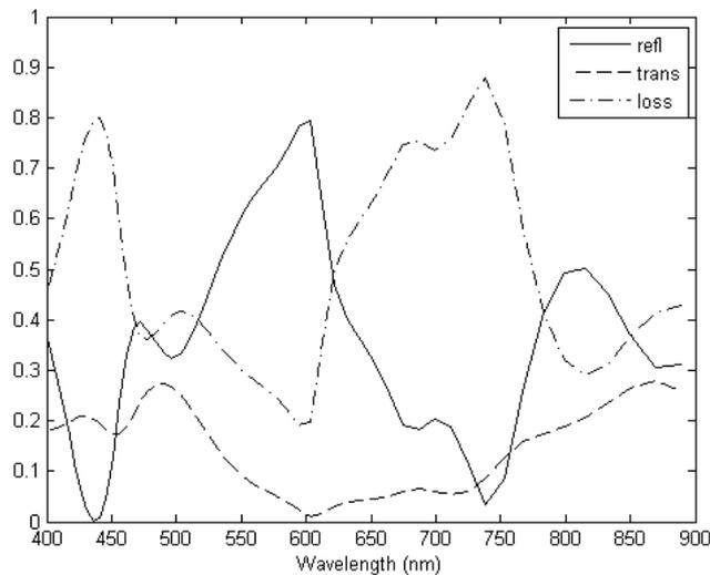
Fig. 3 – Computed reflectance, transmittance, and absorption *versus* the operating wavelength in the proposed structure containing GaAs as absorbing medium with thickness  $d_2 = 120$  nm.
