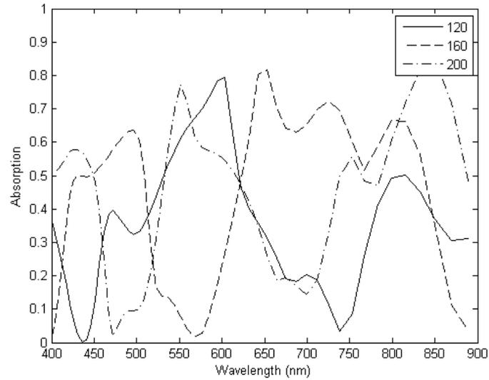
Fig. 4 – Computed absorption spectra of strip waveguide *versus* the operating wavelength for GaAs absorbing materials for different values of  $d_2 = 120, 160,$  and  $200$  nm.
