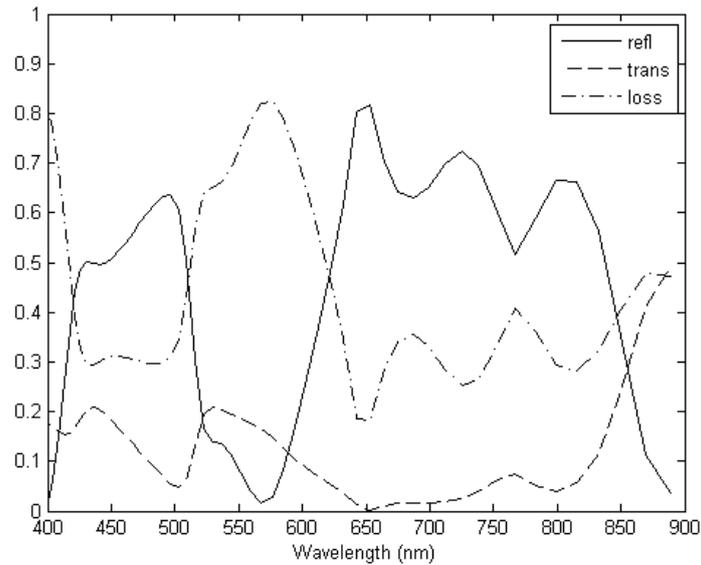
Fig. 2 – Computed reflectance, transmittance, and absorption *versus* the operating wavelength, in the proposed structure containing GaAs as absorbing medium with thickness  $d_2 = 160$  nm.
