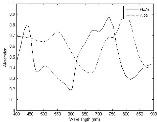
Fig. 5 – Computed absorption spectra of strip waveguide structure *versus* the operating wavelength for two different materials a-Si and GaAs for  $d_2 = 120$  nm.
