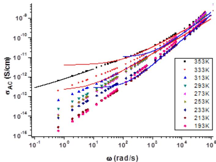
Fig. 1 – (Color online) Frequency dependence of AC conductivity for 20 nm.
