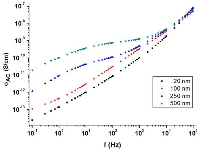
Fig. 5 – Frequency and thickness dependence of AC conductivity at room temperature.
