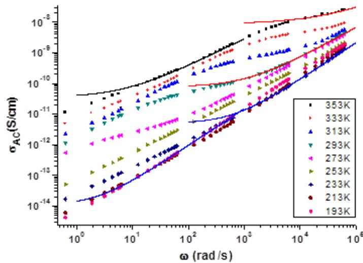
Fig. 3 – Frequency dependence of AC conductivity for 250 nm.
