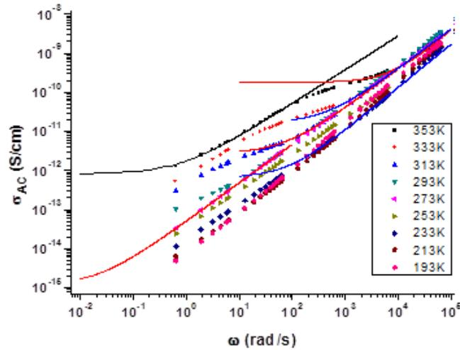
Fig. 2 – Frequency dependence of AC conductivity for 100 nm.
