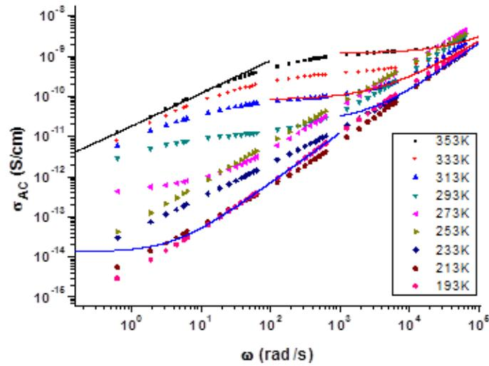
Fig. 4 – Frequency dependence of AC conductivity for 500 nm.
