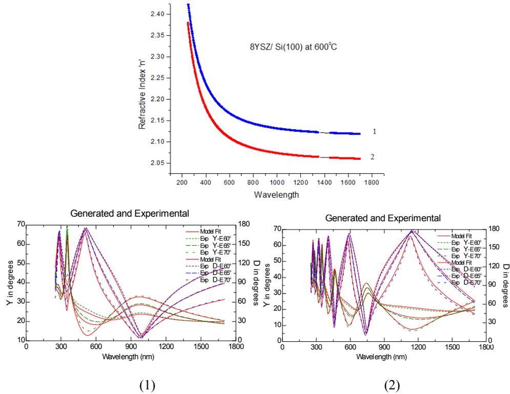
Fig. 5 – Variation of refractive index for 8YSZ/Si (100) for two thin films.
