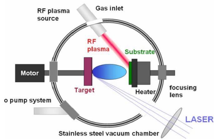
Fig. 1 – A schematic diagram of the pulsed laser deposition setup.
