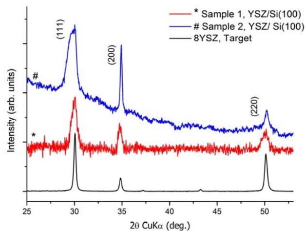
Fig. 2 – XRD spectra of 8YSZ targets, two thin films 8YSZ thin films with different number of pulses.
