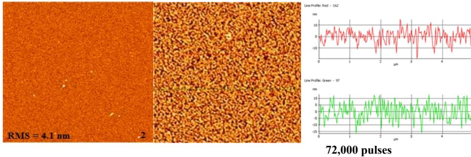
Fig. 4 (continued) – AFM images ( $20 \times 20 \mu\text{m}^2$  and  $5 \times 5 \mu\text{m}^2$ ) areas for two samples of YSZ.
