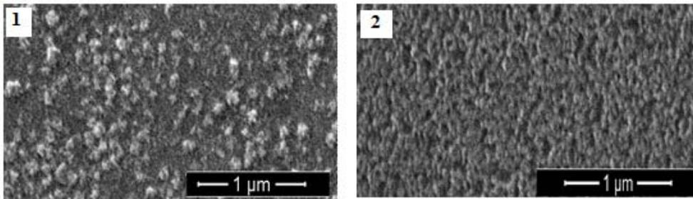
Fig. 3 – SEM for two thin films 8YSZ thin films with 1 with 36,000 pulses and 2 with 72,000 pulses.
