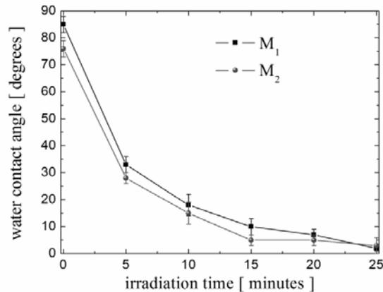
Fig. 4 – Variation of water contact angle for  $TiO_2$  2D patterns obtained by the methods  $M_1$  and  $M_2$ .
