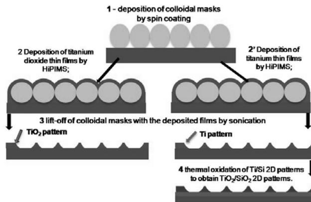
Fig. 1 – Schematic diagram of  $\text{TiO}_2$  nano-pattern fabrication by plasma colloidal lithography using the method  $M_1$  (left side: deposition of CM, reactive m-HiPIMS deposition of  $\text{TiO}_2$  thin films, and mask lift-off), and the method  $M_2$  (right side: deposition of CM, HiPIMS deposition of Ti, mask lift-off and thermal oxidation).
