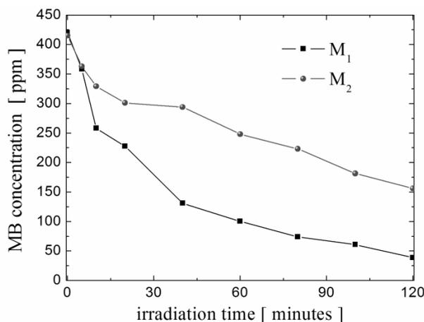
Fig. 5 – Variation of concentration of methylene blue (MB) aqueous solution as result of irradiation with visible light of TiO<sub>2</sub> patterns obtained by the methods M<sub>1</sub> and M<sub>2</sub>.
