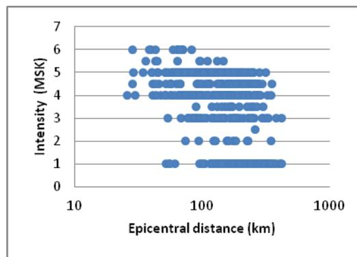
Fig. 6 – The intensity–distance plot for the IDPs obtained for the 25 April 2009 Vrancea subcrustal earthquake.
