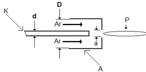
Fig. 3 – Schematic drawing of the plasma source mechanical layout (not in scale). A-anode; K-cathode; P-plasma plume.
