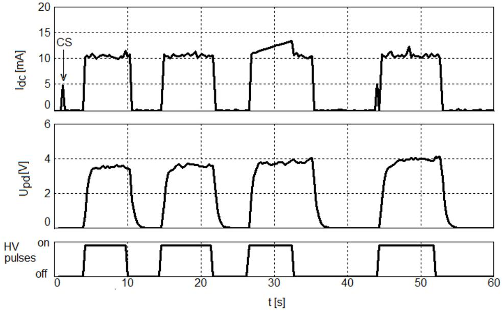
Fig. 4 – Time variation of  $I_{dc}$  and  $U_{pd}$ , if  $|U_{dc}| \approx 495V$ . Experimental conditions:  $R_b = 3k\Omega$ ,  $f=100Hz$ ,  $T_{on}=1ms$ ,  $U_g=3.5V$ .
