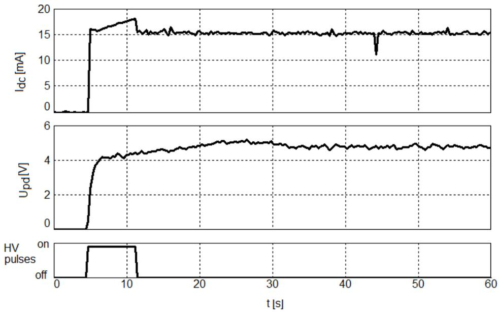
Fig. 5 – Time variation of  $I_{dc}$  and  $U_{pd}$ , if  $|U_{dc}| \approx 590V$ . Experimental conditions:  $R_b = 3k\Omega$ ,  $f=100Hz$ ,  $T_{on}=1ms$ ,  $U_g=3.5V$ .
