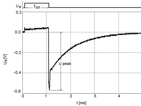
Fig. 2 – Top trace: Waveform of the excitation voltage  $U_e$ . Bottom trace: Waveform of a high voltage pulse recorded by a digital oscilloscope connected to point D.  $U_{peak} \approx -0.57V$  corresponds to output pulse voltage peak value  $\approx -3.88kV$ . Experimental conditions:  $U_{dc}=0$  (no plasma)  $U_g=2V$ ,  $f=100Hz$ ,  $T_{on}=1ms$ .
