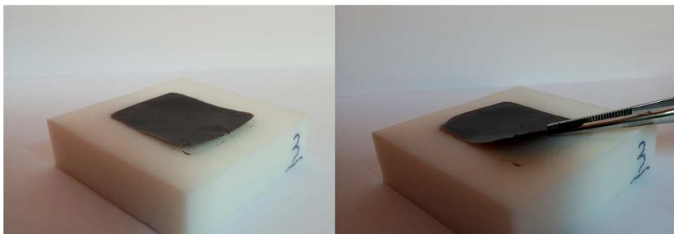
Fig. 1 – The process of obtaining graphene oxide freestanding film
