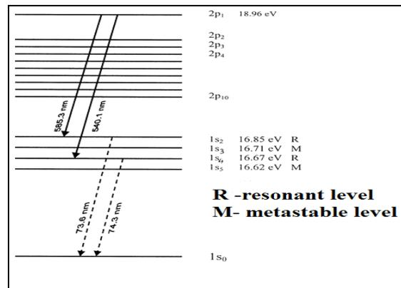
Fig. 3 - Simplified Paschen energy diagram of neon.
