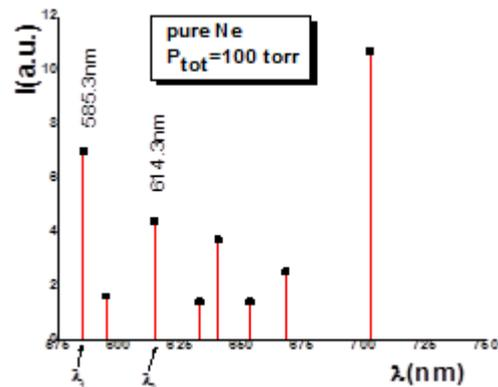
Fig. 4 — Emission spectrum of DBD discharge in pure Neon.
