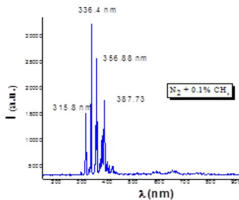
Fig. 7- Emission spectrum of (nitrogen+0.1% methane) gas mixture plasma in d.c. flowing discharge (p=4 mbar, I=50 mA).
