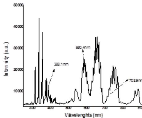
Fig. 6 - Emission spectrum of pure molecular nitrogen plasma in d.c. flowing discharge (p=4 mbar, I=50 mA).
