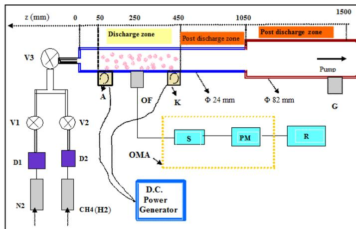
Fig. 2 - Experimental set-up of the nitrogen/hydrogen gas mixture plasma in d.c. flowing discharge (D1, D2 – flow meters; V1, V2, V3 – valves; S - spectrophotometer; PM – photomultiplier; R- recorder; OF – optical fiber; G- thermal gauge, A - anode, K- cathode, OMA- Optical Multichannel Analyzer).
