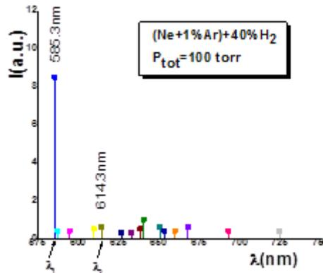
Fig. 5 — The emission spectrum of DBD discharge in (Ne+40% H<sub>2</sub>) gas mixture.
