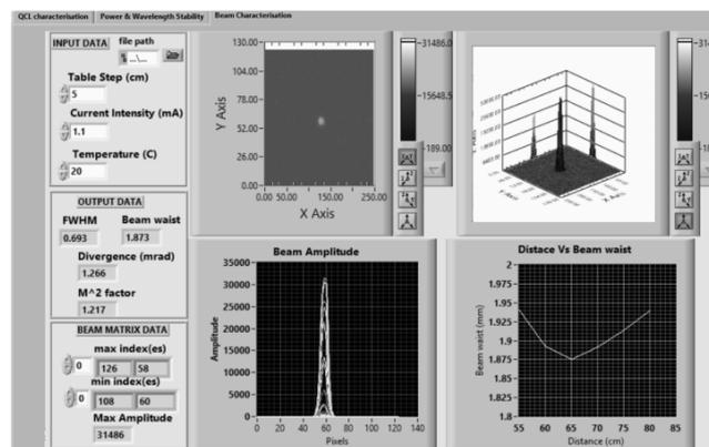
Fig. 5 – Example of a QCL beam characterization.
