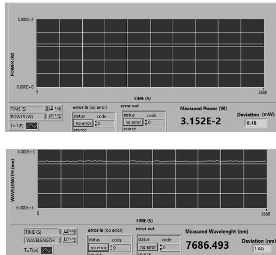
Fig. 4 – Example of optical power and wavelength stability measurements.
