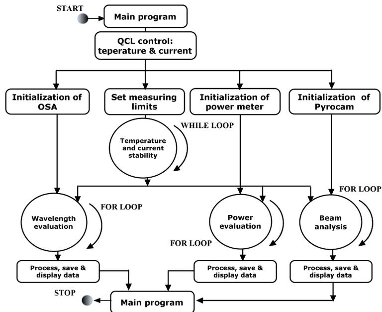
Fig. 2 – Flow chart of the LabVIEW program used for the QCL characterisation.
