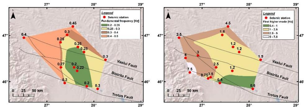
Figure 4. Variation of fundamental frequency (left) and the first higher peak(right) over the area under investigation.
