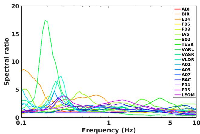
Figure 3. H/V spectral ratios of ambient vibrations at each station in the Moldavian and Scythian Platforms.
