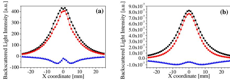
Fig. 5 – (a) Measured backscatter power distributions from the investigated host medium ( $C_h = 0.406\%$  IL) with (red circles) and without (black squares) inhomogeneity ( $C_i = 2.067\%$  IL) and their difference (inhomogeneity image, blue triangles - see Fig. 4,  $z_s = 0$ ). (b) Theoretical curves (and their difference, blue triangles) of  $J(x, y_c)$  for  $C = 2.067\%$  IL (red circles) and  $0.406\%$  IL (black squares) evaluated on the basis of Eq.(A.1) at  $g = 0.865$ .
