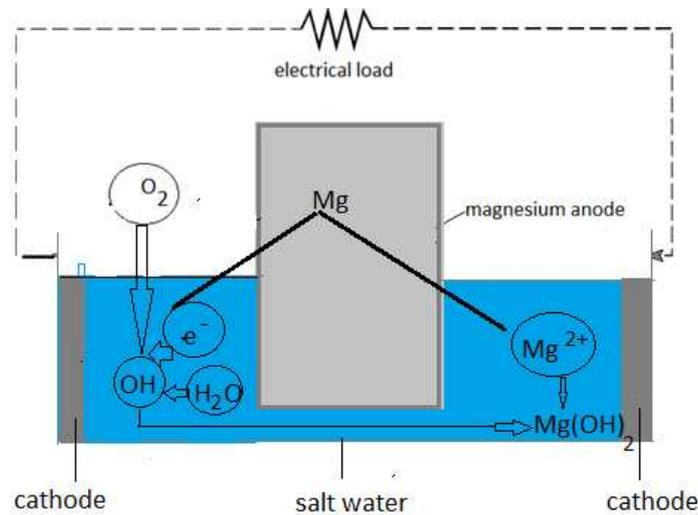
Fig. 3 – The working principle of the magnesium fuel cell with salt water. The colored versions can be accessed at <http://www.infim.ro/rrp/>.
