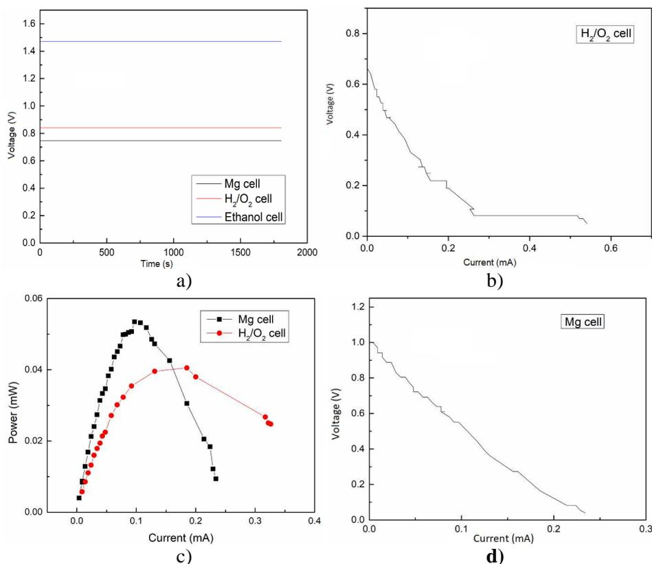
Fig. 7 – Examples of curves recorded by the monitoring system: a) open circuit voltage on time; b) polarization curve for H<sub>2</sub>/O<sub>2</sub> cell; c) power curves; d) polarization curve for Mg cell. The colored versions can be accessed at <http://www.infim.ro/rfp/>.
