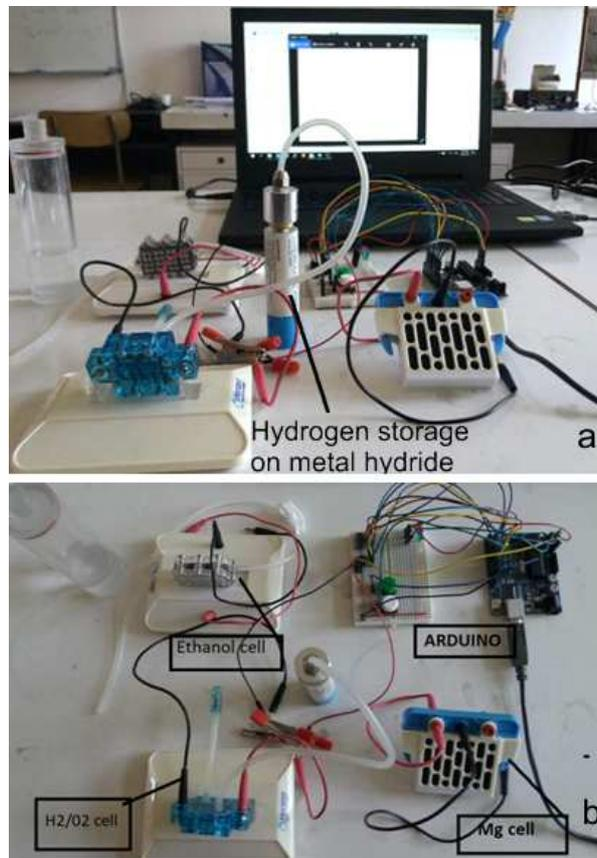
Fig. 6 – Laboratory setup for experimental tests a) monitoring system; b) system of fuel cells and Arduino microcontroller. The colored versions can be accessed at <http://www.infim.ro/rrp/>.
