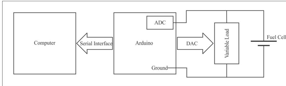
Fig. 4 - Developed monitoring system architecture.
