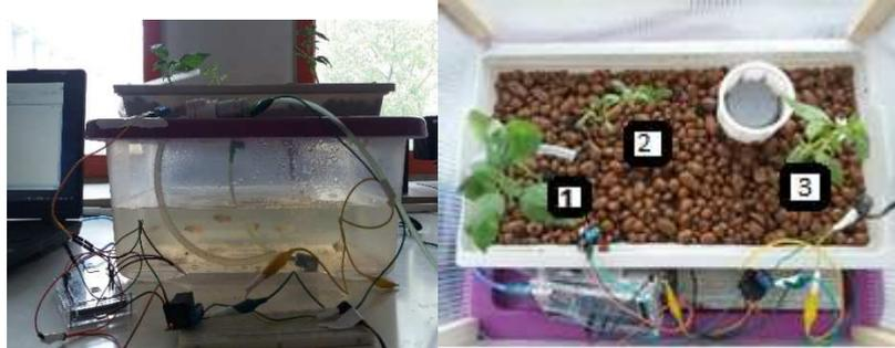
Fig. 9 – The experimental aquaponics system with fishes and plants (basil 1,2,3). The colored versions can be accessed at <http://www.infim.ro/rp/>.
