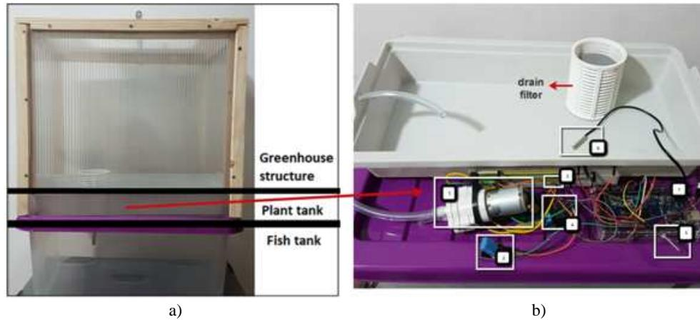
Fig. 8 – The experimental aquaponics system: a) structure of aquaponics system; b) monitoring system 1 - water pump, 2 - temperature and humidity sensor, 3 - resistance 10 k $\Omega$ , 4 - relay, 5 - light sensor, 6 - analog temperature sensor, 7 - Arduino Mega 2560. The colored versions can be accessed at <http://www.infim.ro/rfp/>.
