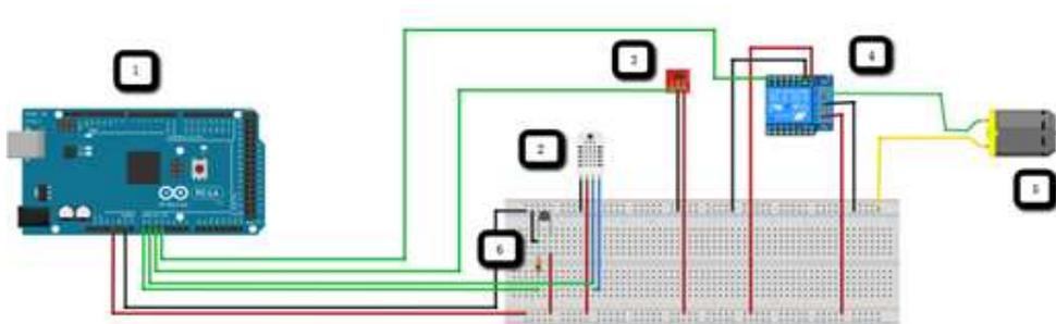
Fig. 6 – Electric scheme of monitoring system: 1 - Arduino Mega 2560, 2 - temperature and humidity sensor DHT11, 3 - light sensor, 4 - 5V relay, 5 - DC motor (water pump simulation), 6 - analogue temperature sensor. The colored versions can be accessed at <http://www.infim.ro/rfp/>.
