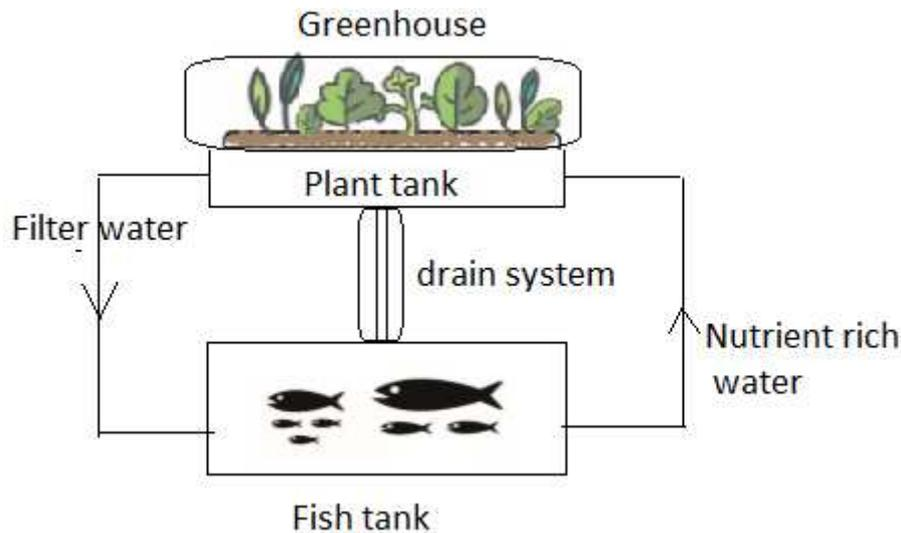
Fig. 1 – The schematic aquaponics system. The colored versions can be accessed at <http://www.infim.ro/rfp/>.
