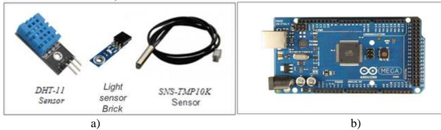
Fig. 3 – Components of the monitoring system: a) Data acquisition unit; b) Arduino unit. The colored versions can be accessed at <http://www.infim.ro/rfp/>.
