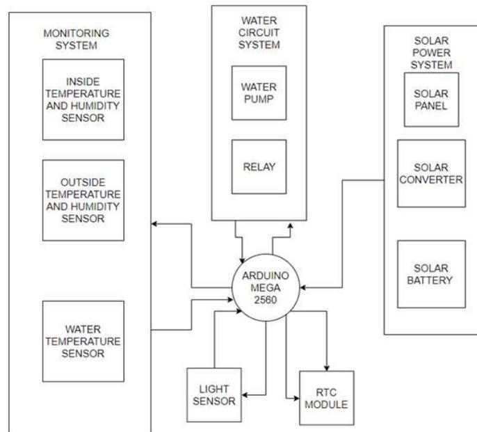
Fig. 7 – Assembly scheme of aquaponics system.
