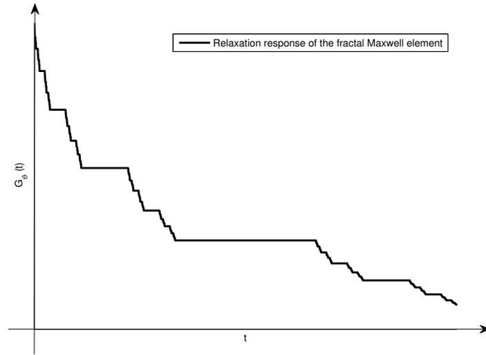
Fig. 5 – The relaxation response of the fractal Maxwell element for  $\vartheta = \ln 2 / \ln 3$ .
