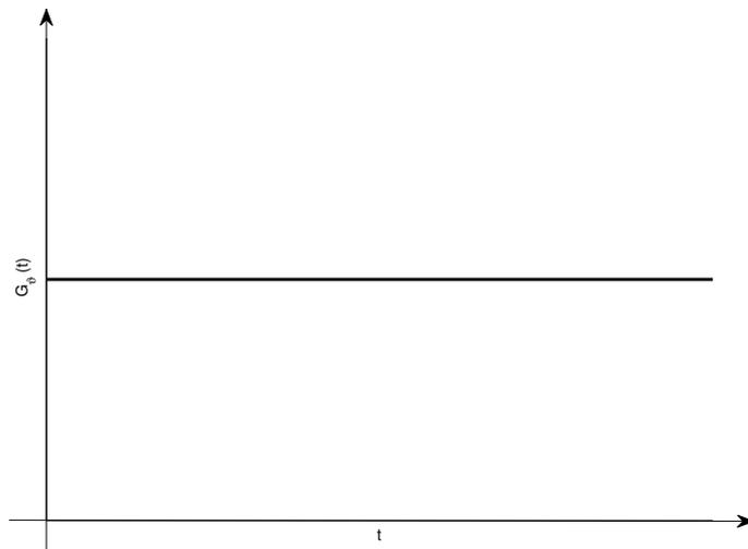
Fig. 8 – The relaxation response of the fractal Kelvin-Voigt element for  $\vartheta = \ln 2 / \ln 3$ .
