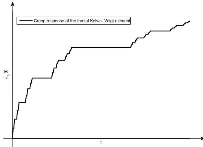
Fig. 7 – The creep response of the fractal Kelvin-Voigt element for  $\vartheta = \ln 2 / \ln 3$ .
