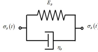
Fig. 6 – The representation of the fractal Kelvin-Voigt element involving LFD.
