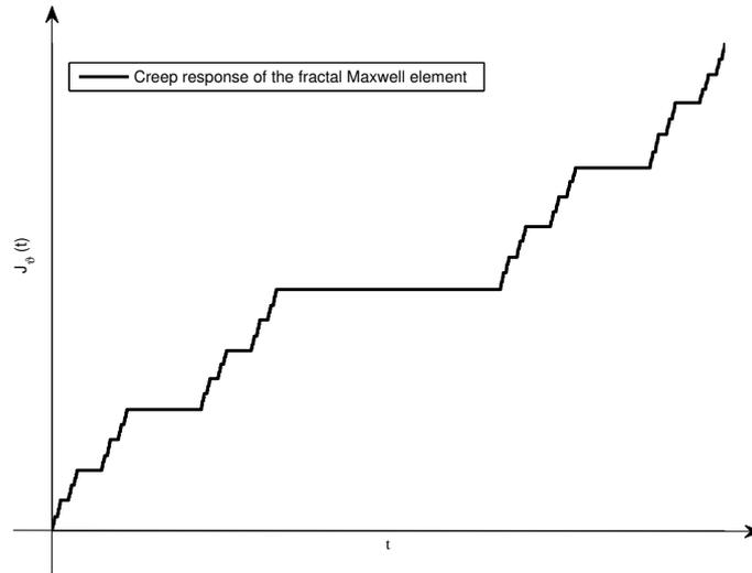
Fig. 4 – The creep response of the fractal Maxwell element for  $\vartheta \ln 2 / \ln 3$ .
