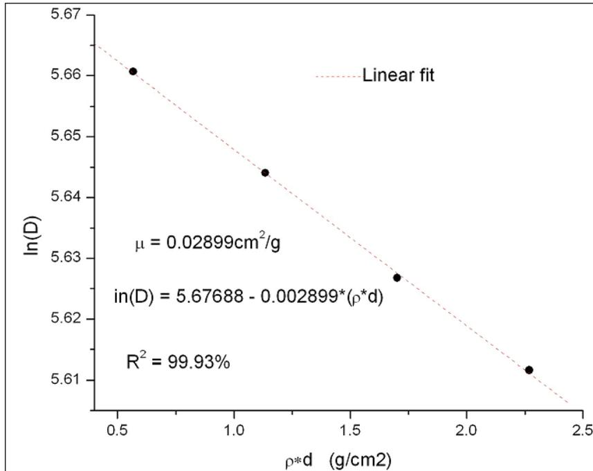
Fig. 1 – Experimental  $\ln(D)$  variation as a function of absorber thickness.
