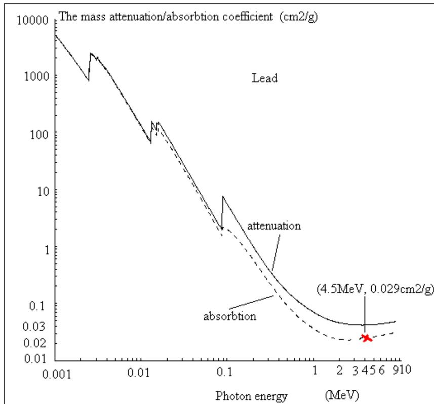
Fig. 2 – Attenuation/absorption coefficient as a function of energy.
