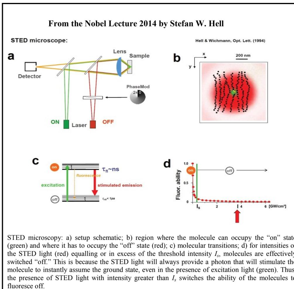
Fig. 2 – Scheme of the principles of STimulated Emission Depletion-microscopy (STED).
