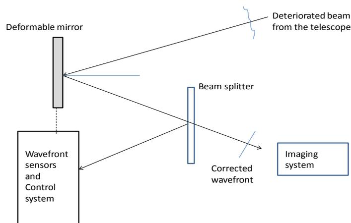
Fig. 3 – Scheme of adaptive optics procedure.
