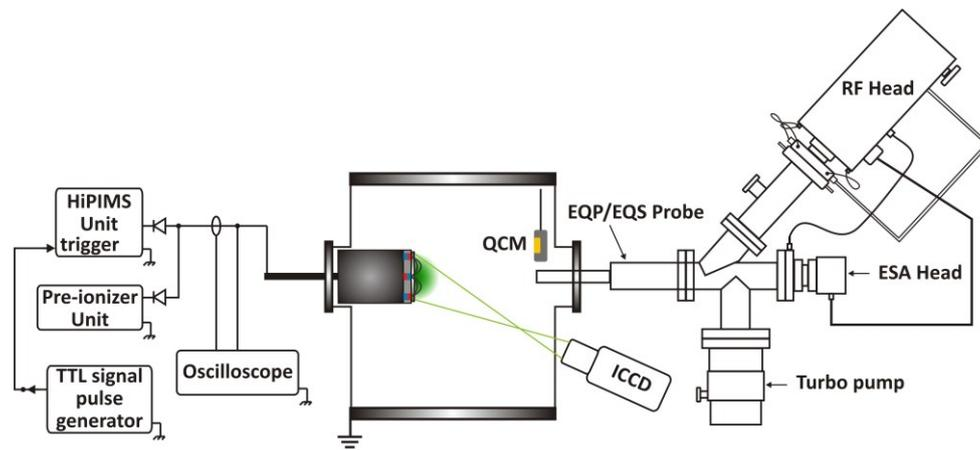
Fig. 1 – Schematic view of the experimental setup including the HiPIMS system, quartz crystal microbalance (QCM), ICCD camera (ICCD), and mass spectrometer.
