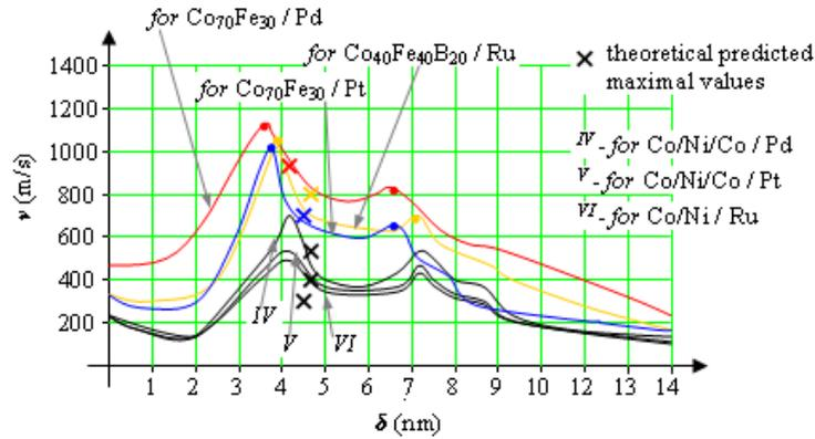
Fig. 2 – Evolution of the DW velocity in function of the dynamic domain with  $\delta$  for the considered materials, for a level of excitation of:  $H=1.2$  kOe and  $j_c = 0.5 \cdot 10^{12}$  A/m<sup>2</sup>.
