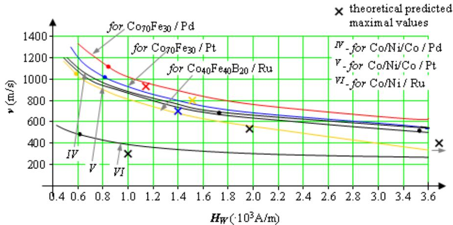
Fig. 3 – Evolution of the DW velocity in function of the Walker breakdown field  $H_W$  for the considered materials, for a level of excitation of:  $H=1.2$  kOe and  $j_c = 0.5 \cdot 10^{12}$  A/m<sup>2</sup>.
