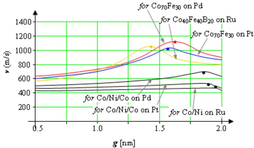
Fig. 5 – Dependence of the DW velocity on the nanometric thickness of the grain size  $g$  in the polycrystalline magnetic thin film. Velocity maxima obtained in graphs in Fig. 2 (colored circles) can be observed in the peak zone of the curves represented here.
