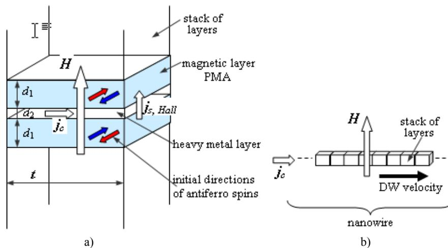
Fig. 1 – a) The active stack of layers: two PMA antiferro layers are joined by a ultrathin heavy metal layer. The directions of the applied field  $H$  and propagation current  $j_c$  are indicated and also the generated spin Hall current; b) nanowire in the racetrack memory.
