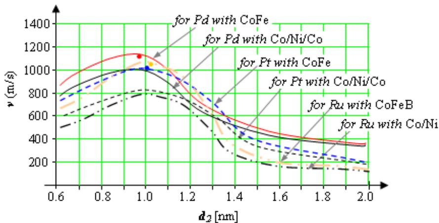
Fig. 4 – Dependence of the DW velocity on the nanometric thickness of the heavy metal layer  $d_2$ , which represent a control parameter of the structure. Velocity maxima obtained in graphs in Fig. 2 (colored circles) can be observed in the peak zone of the curves represented here.
