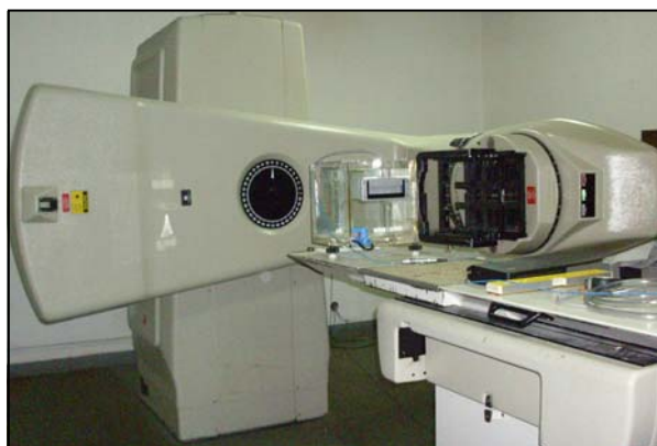
Fig. 1 – The Co-60 radiotherapy device Theratron 1000E type, of Radiotherapy Laboratory – IOB.
