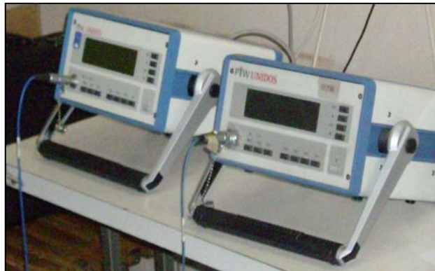
Fig. 2 – The UNIDOS PTW dosimeters used for measuring air kerma and absorbed dose to water.
