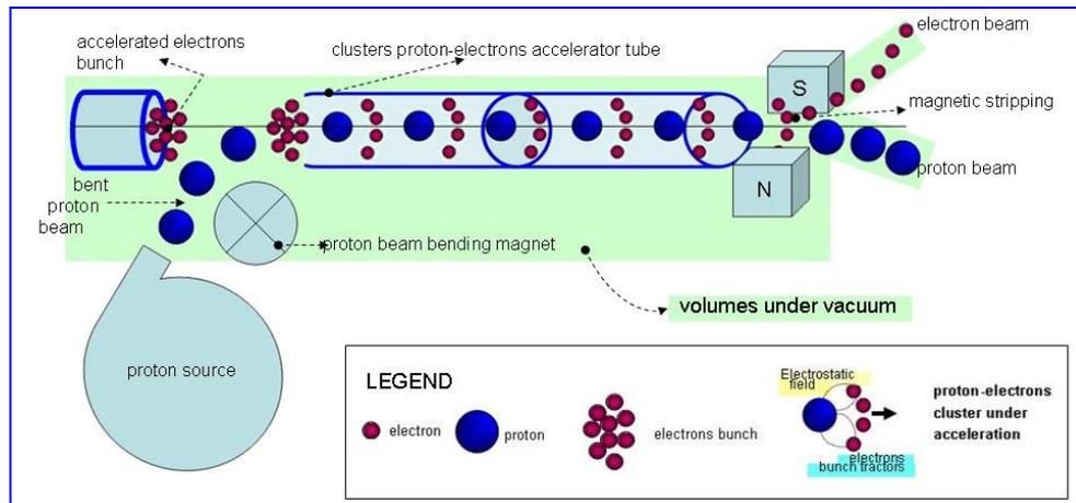
Fig. 4 – The schematic representation of the second step of accelerating protons by using electrons.
