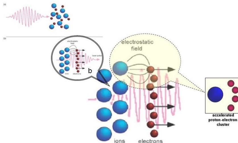
Fig. 2 – TNSA, generation of electrons and ions [14] with the electrostatic field created between them – a schematic representation [14].
