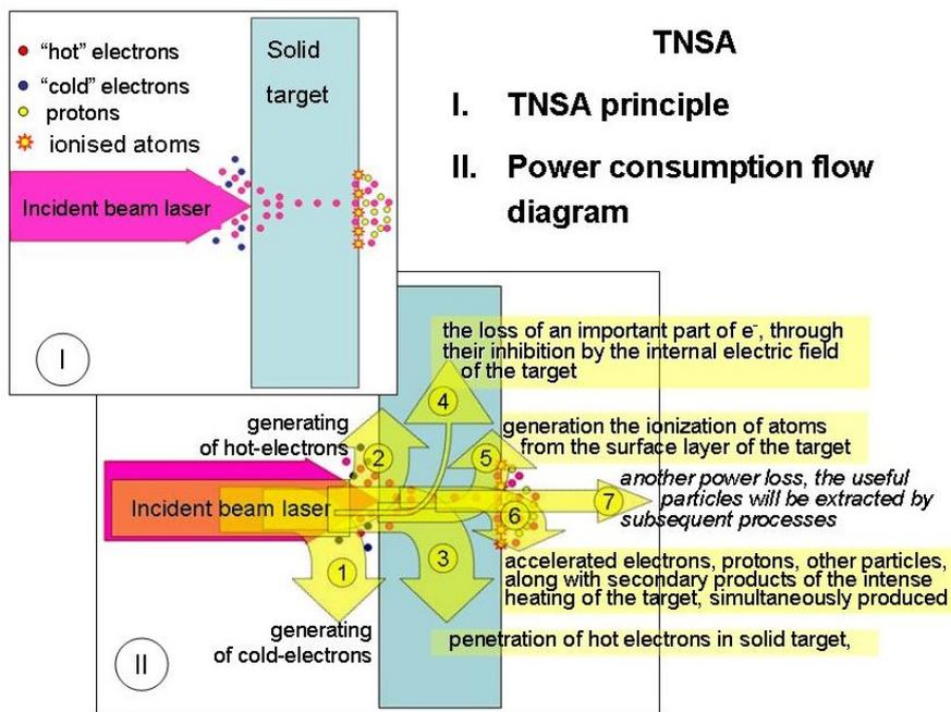
Fig. 1 – Schematic representation of the TNSA mechanism and the corresponding laser beam power consumption flow diagram [15, 16].
