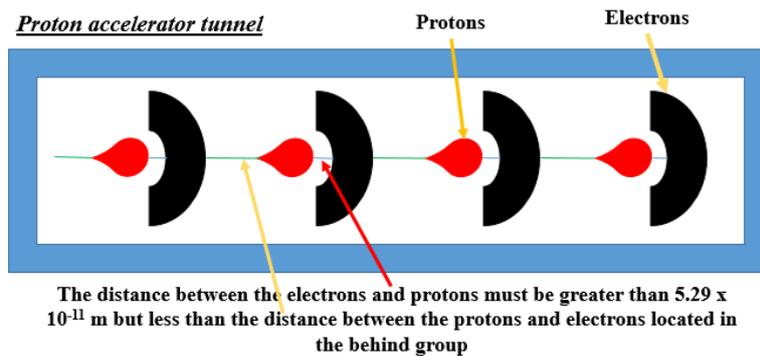
Fig. 5 – Groups of GeV electrons and protons on the accelerator tunnel. The relevant geometrical distances are shown.
