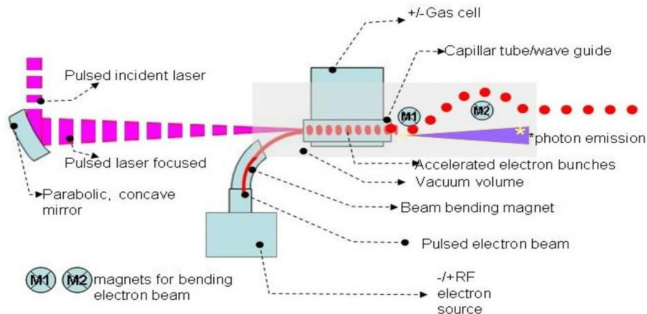
Fig. 3 – Schematic representation of the LWFA-based accelerator in the two versions discussed in the text. By using the external electron source the gas cell is no longer needed simplifying the acceleration model [12, 13 and 8]. See text for details.
