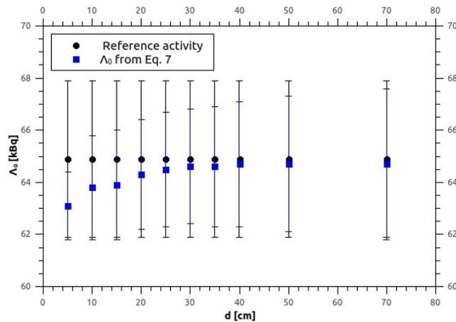
Fig. 5 – The dependence of the calculated activity  $\Lambda_0$  as a function of the distance.
