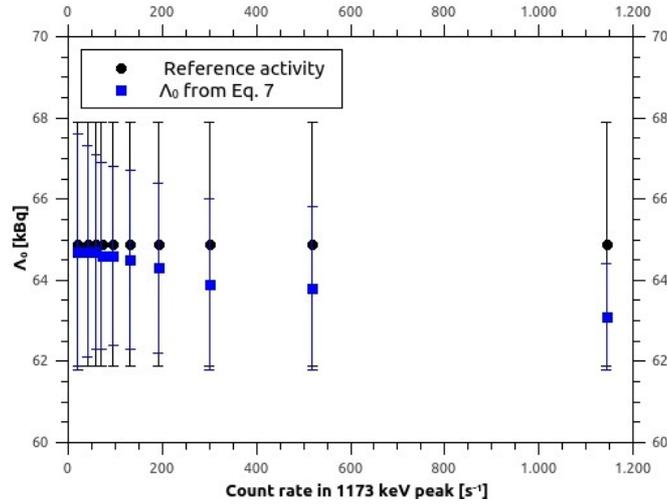
Fig. 6 – The dependence of the calculated activity  $\Lambda_0$  as a function of the count rate in the 1173 keV peak. The correct value of the activity  $\Lambda$  is given by the asymptotic value of the  $\Lambda_0$  for  $N_1$  approaching zero.
