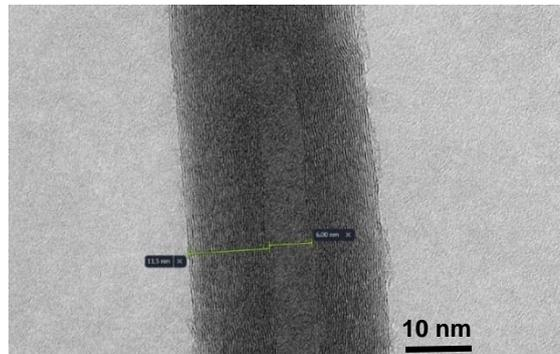
Fig. 3 – HR-TEM image of an individual MWCNT.
