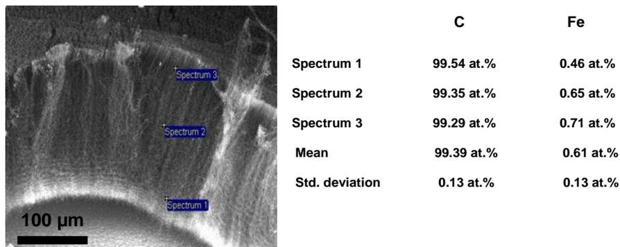
Fig. 2 – EDX analysis in three points along the vertically aligned MWCNT array.
