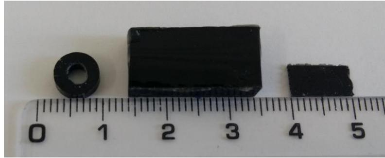
Fig. 1 – MWCNT/Co-Fe-B composite material in different shapes.
