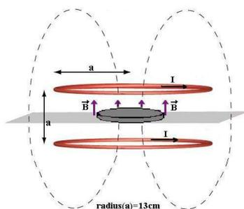
Fig. [1.] - Schematic drawing of the MF exposure system of mushroom samples; B — magnetic flux density; I — current intensity; a — radius of coil from Helmholtz coil system.
