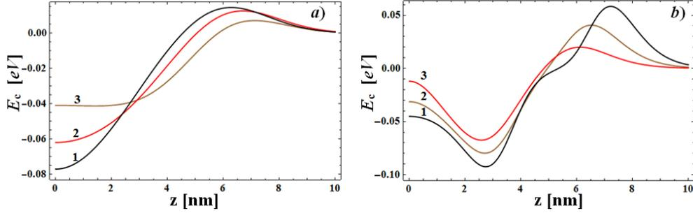
Fig. 6 – The coordinate dependence of the bottom of the conduction band at  $N_0 = 5 \cdot 10^{19} \text{ cm}^{-3}$
