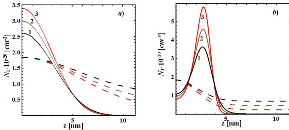
Fig. 4 – The spatial distribution of interstitial atoms of zinc ( $N_0 = 10^{19} \text{ cm}^{-3}$ ) at different values of the depth of radiation absorption and substrate temperature:
