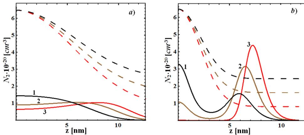
Fig. 5 – The spatial distribution of oxygen vacancies ( $N_0 = 10^{19} \text{ cm}^{-3}$ ) at different values of the depth of radiation absorption and substrate temperature:
