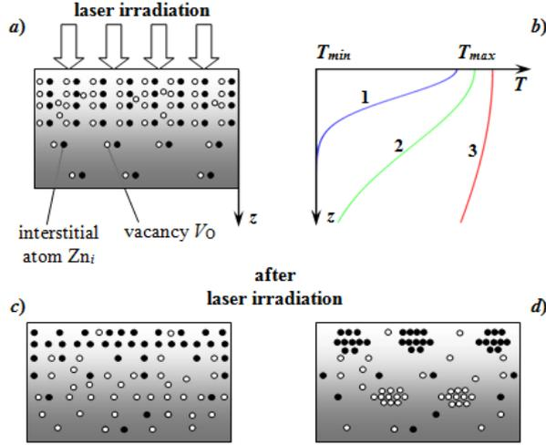
Fig. 1 – The geometric model of ZnO semiconductor exposed to laser irradiation (a), and the spatial distribution of the temperature in the depth of the crystal (b); the geometric model of semiconductor after laser irradiation (the clusters of defects are not formed (c), the clusters of defects are formed (d).
